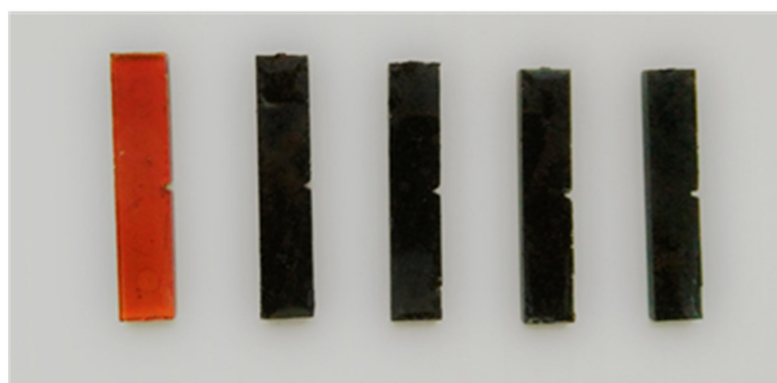
Figure 7. The test samples for the mechanical properties and impact resistance tests. Photographs from left to right are 0, 0.5, 1, 2, and 2.67 wt.% of AMG nanosheets addition.
