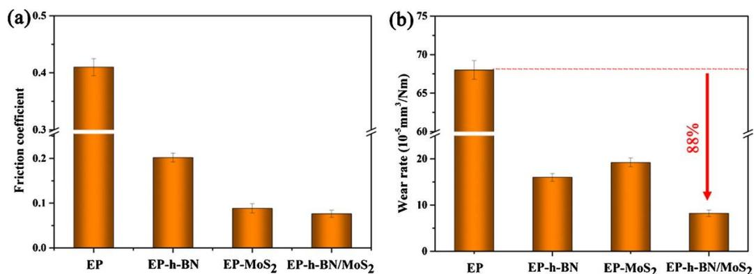
**Figure 10.** (a) Coefficient of friction and (b) wear rate of EP, EP-h-BN, EP-MoS<sub>2</sub> and EP-h-BN/MoS<sub>2</sub> composite coatings sliding against 440c ball under dry friction (EP = epoxy). Reproduced with permission from [102]. Copyright 2010 Elsevier.
