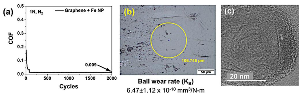
**Figure 9.** Iron nanoparticles mixed with graphene flakes and sliding against the hydrogenated diamond-like-carbon surface: (a) COF ( $0.0087 \pm 0.0008$ ) and (b) DLC ball wear diameter and estimated ball wear rate. (c) TEM image of wear debris collected from the wear track after 500 wear cycles, revealing a well-formed onion-like carbon nanostructure. Reproduced with permission from [84]. Copyright 2019 John Wiley and Sons.
