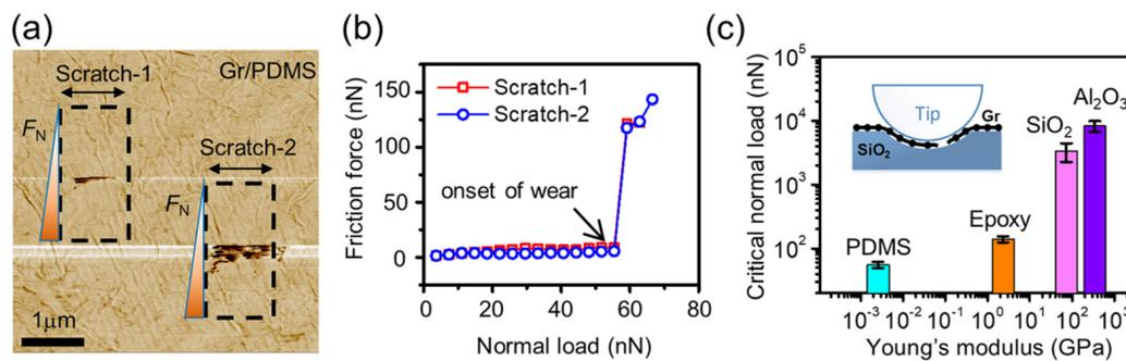
**Figure 3.** (a) A lateral force image of graphene/PDMS sample done under a low load after two scratch tests; the black arrows indicate the scratch direction. (b) Variations of friction with the normal load during the scratch tests in (a). (c) Critical normal loads of graphene on the substrates with different stiffnesses. Reproduced with permission from [67]. Copyright 2019 AIP Publishing.
