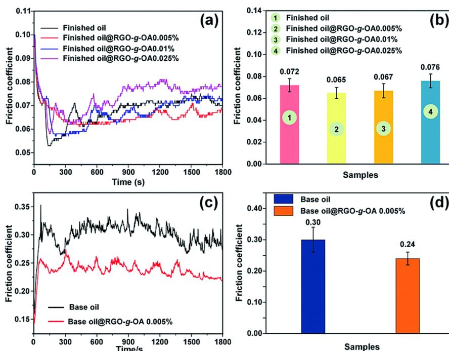
**Figure 8.** (a,c) Typical friction coefficients with time and (b,d) average friction coefficients of pristine finished oil, base oil and the ones filled with various mass contents of RGO-g-OA on steel discs; the load applied is 100 N. Reproduced with permission from [61]. Copyright 2019 Royal Society of Chemistry.
