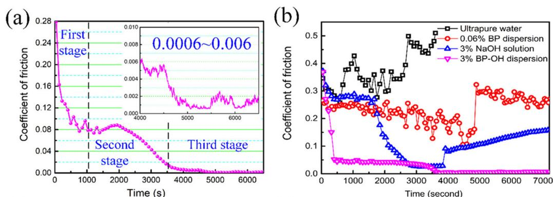
**Figure 12.** (a) Variation in the COF with time using the 7 wt.% BP-OH aqueous solution as the lubricant. The inset is the magnified graph of the COF after the running-in period. (b) The comparative plots of the COFs of four different lubricants including ultrapure water, 3% NaOH solution, 0.06% BP Dispersion and 3% BP-OH dispersion. Reproduced with permission from [119]. Copyright 2018 American Chemical Society.
