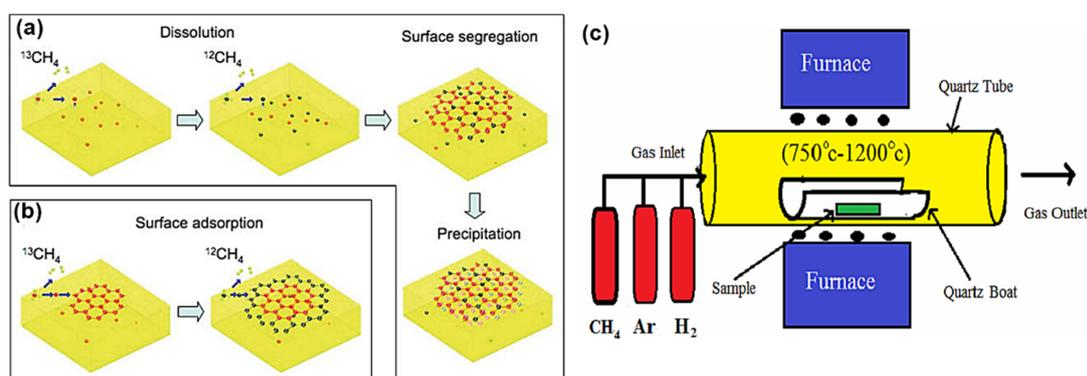
**Figure 2.** (a,b) Schematic demonstration of the growth mechanism of graphene. Reproduced with permission from [57]. Copyright 2009 American Chemical Society. (c) Schematic illustration of the CVD process setup. Reproduced with permission from [58]. Copyright 2015 CSIR-NISCAIR.
