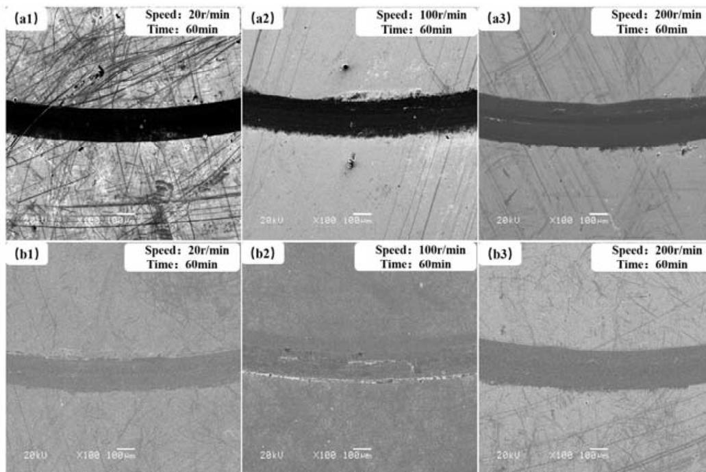
**Figure 11.** The morphologies of the wear tracks for pure MoS<sub>2</sub> film (a1–a3) and the MoS<sub>2</sub>–WS<sub>2</sub> composite film (b1–b3) after atomic oxygen irradiation at varying sliding speeds. Reproduced with permission from [111]. Copyright 2020 MDPI AG.
