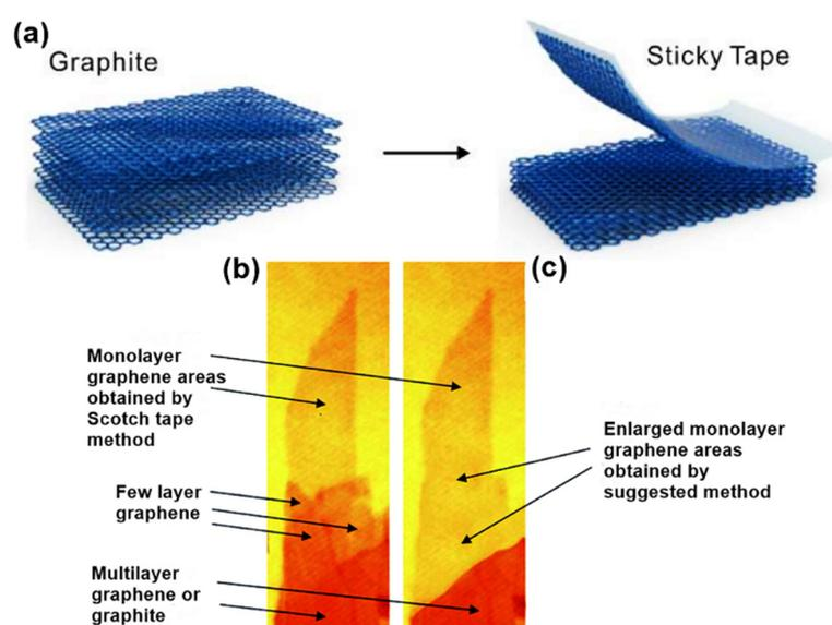
**Figure 1.** (a) Schematic illustration of the mechanical exfoliation of monolayer graphene [49]. Optical images of monolayer graphene (b) as-prepared by scotch tape method and (c) as enlarged using Shmavonyan suggested method. Reproduced with permission from [46]. Copyright 2013 National Academy of Sciences of Armenia.
