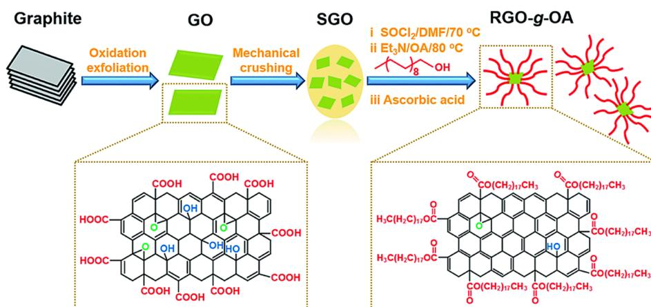
**Figure 7.** Schematic of preparation procedures for RGO-g-OA. Reproduced with permission from [61]. Copyright 2019 Royal Society of Chemistry.
