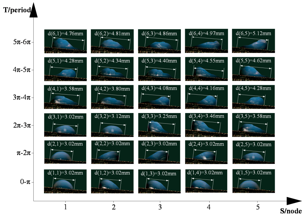
Figure 3. Transient evolution of vibrating drop in three periods on textured surfaces.
