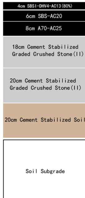
Figure 2. The STR9 structure of RIOHTrack full-scale track.
