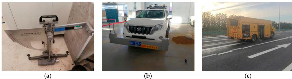
**Figure 4.** Testing equipment for skid resistance of RIOHTrack full-scale track. (a) BM-III British pendulum tester, (b) multi-function testing vehicle (CISC III), (c) sideway force coefficient measuring vehicle.
