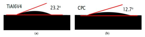
Figure 8. Contact angle measurements (a) on titanium alloy substrate; (b) on CPC coating (S5).
