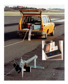
**Figure 1.** The VTI stationary profilometer, with its "macro" sensor mounted on the sled, and the "micro" sensor inserted in the photo, resized to approximately 5 times the scale of the rest of the photo. The photo was shot in another project.
