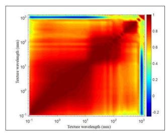
**Figure 4.** Intercorrelation between texture wavelength bands. The correlation coefficient values are illustrated by color according to the scale on the right.
