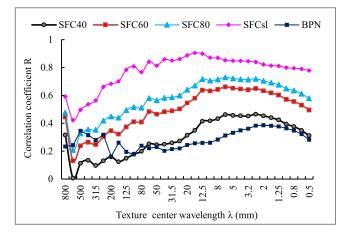
**Figure 5.** The correlation between friction values and road texture wavelength (*SFC*40 represents *SFC* at 40 km/h; *SFC*60 represents *SFC* at 60 km/h; and *SFC*80 represents *SFC* at 80 km/h).
