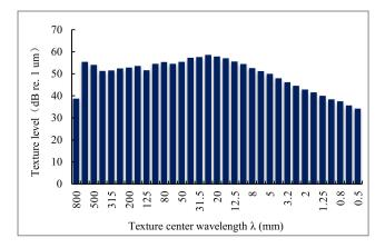
**Figure 2.** An example of a texture third-octave band spectrum (test site 1, a very rough chip seal). In this study, 95 % confidence limits were within  $\pm 1.5$  dB in the range 2–100 mm and within  $\pm 2.5$  dB at the longer and shorter wavelengths.
