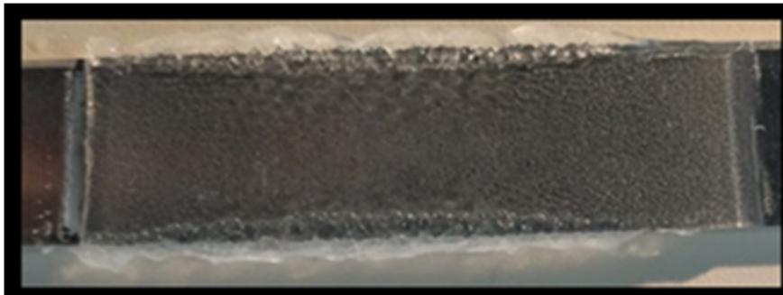
**Figure 17.** Image of glaze ice obtained in the IWT on a flat sample.
