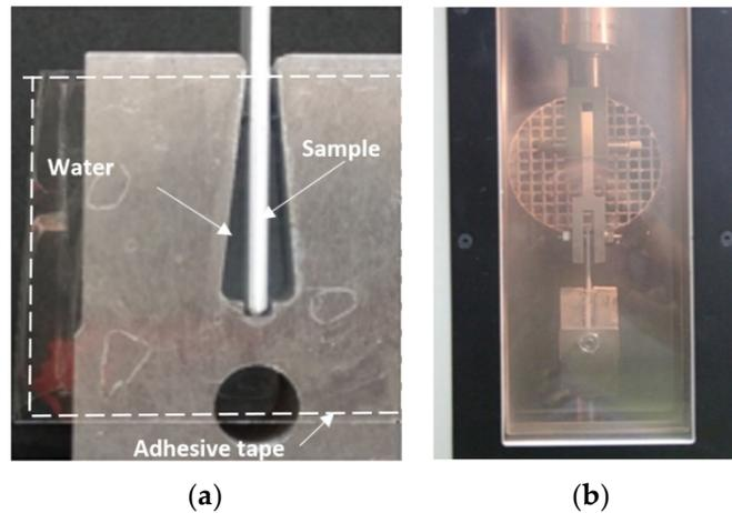
**Figure 6.** (a) Test block employed to form ice on both sides of the sample. (b) Block attached to the Universal machine ready to start a test.
