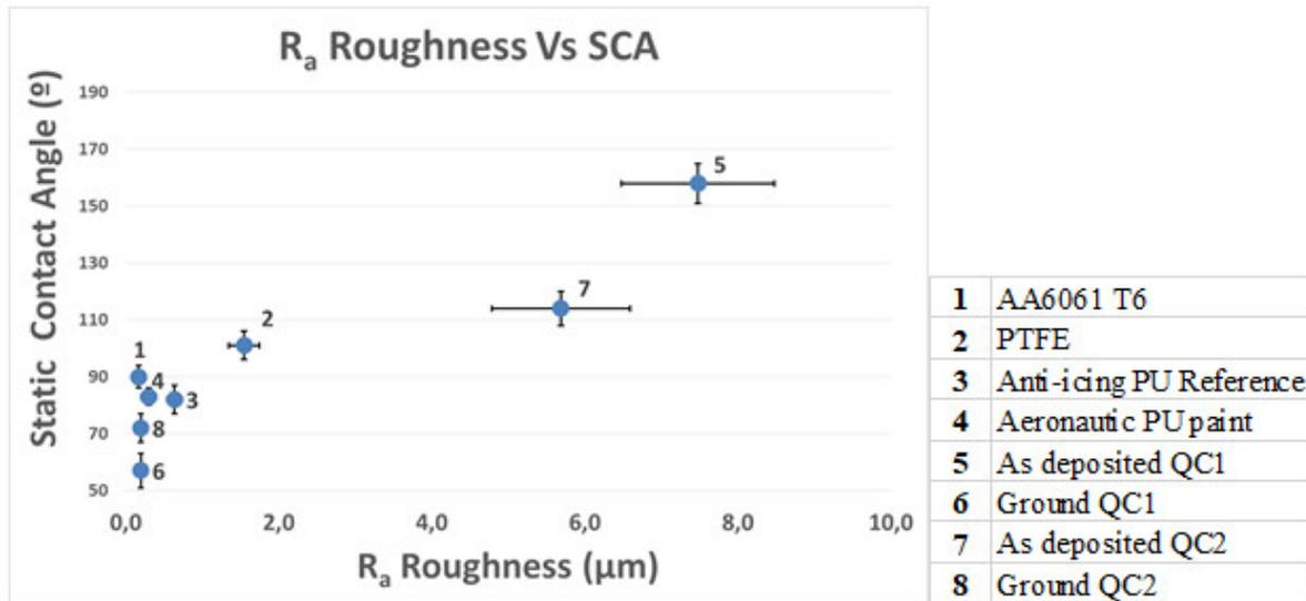
Figure 13. SCA vs  $R_a$  roughness for the studied materials and coatings.
