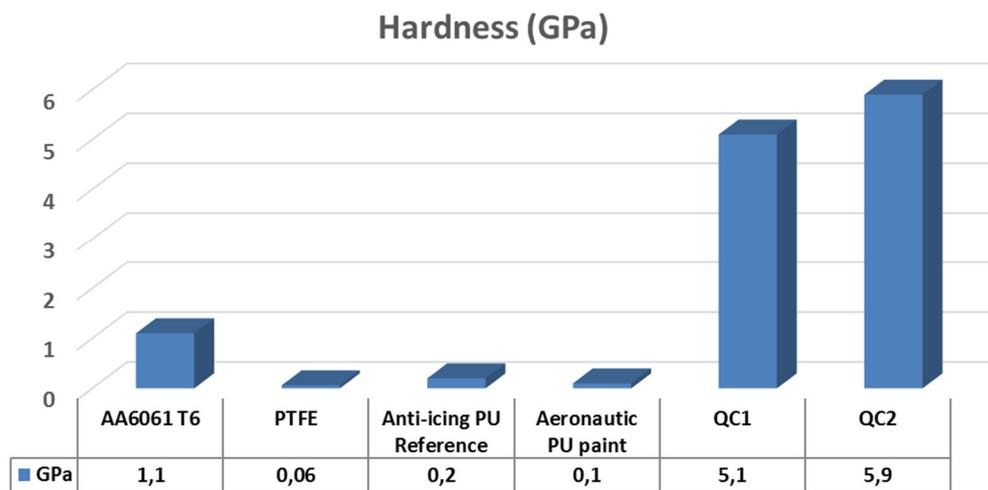
Figure 8. Vickers microhardness measured in all tested materials.
