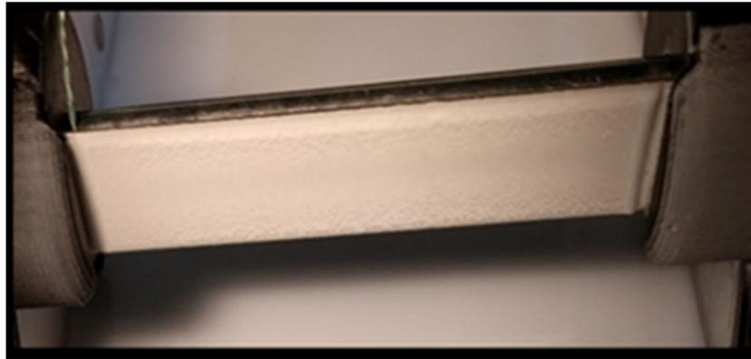
Figure 15. Image of rime ice obtained in the IWT on flat sample profiles.
