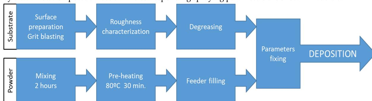
**Figure 3.** Scheme of the previous processes to HVOF deposition.
