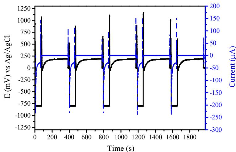
**Figure 2.** Time-potential-current curves for the first five cycles of underpotential deposition (UPD)-Mn and surface-limited redox replacement (SLRR)-Cu.
