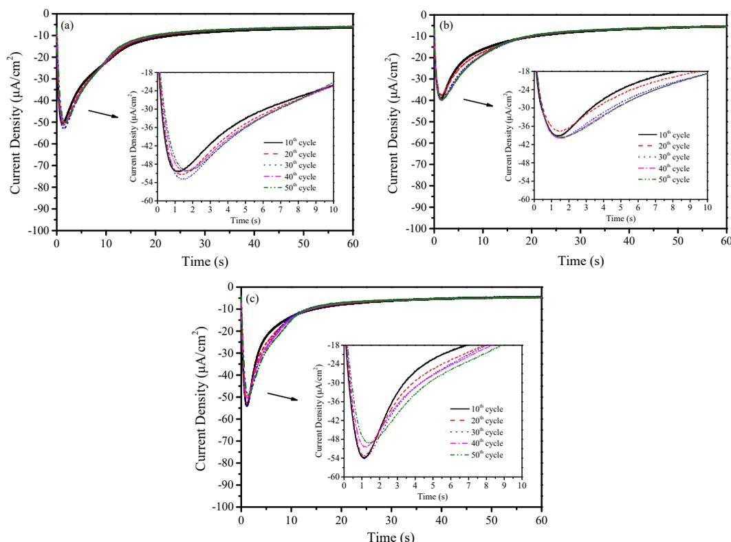
**Figure 3.** Current density–time curves for the UPD-Mn deposited at  $-800$  mV for 60 s, and that were subsequently replaced by  $Cu^{2+}$  during the Cu-SLRR, terminated at a time of (a) 60 s, (b) 40 s, and (c) 20 s.
