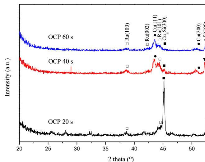
**Figure 8.** XRD results for the Cu(Mn) films annealed at 600 °C.
