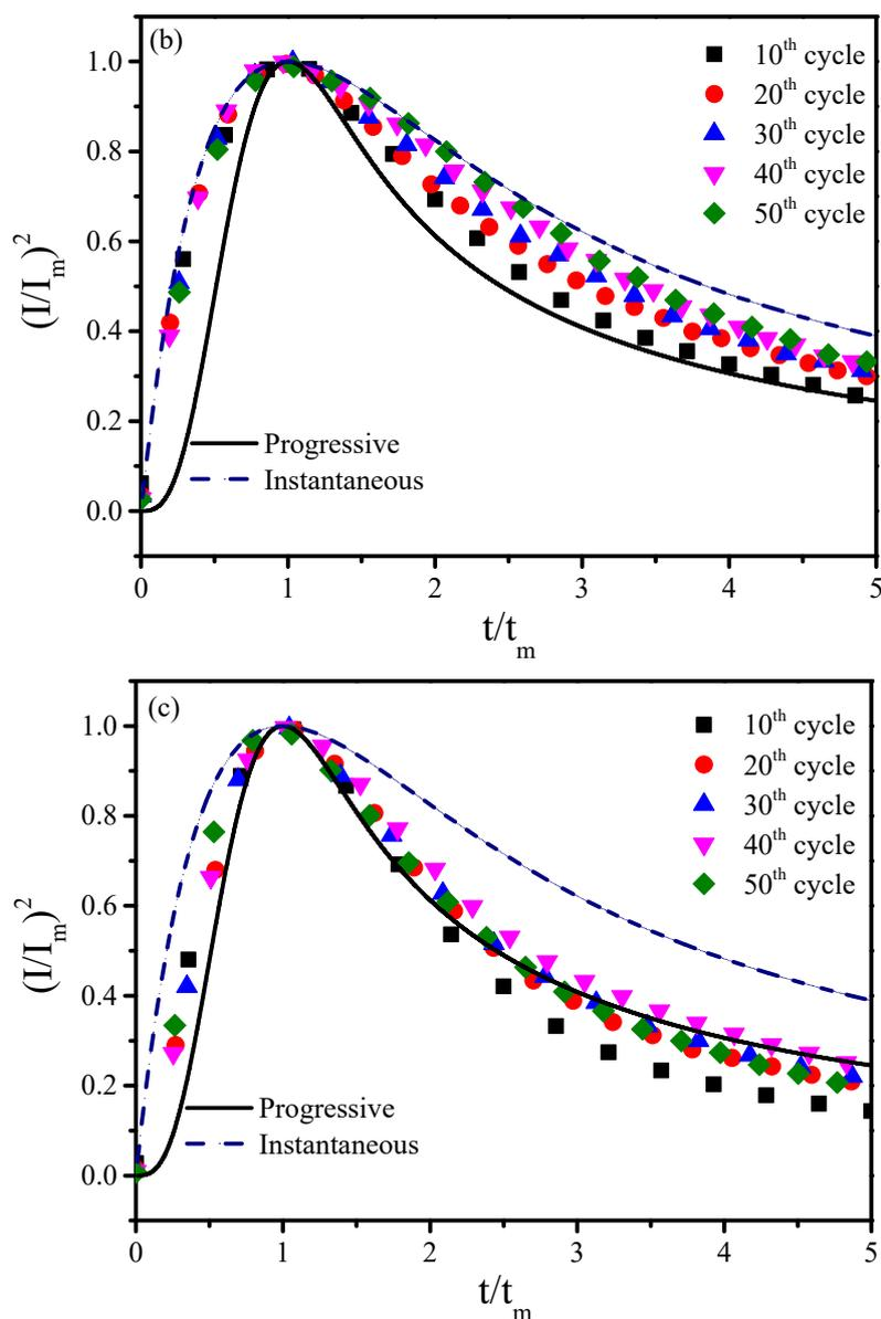
**Figure 4.**  $(I/I_m)^2$  vs.  $t/t_m$  curves for the UPD-Mn in the electrolytes, with various terminated open circuit potential (OCP) times of (a) 60 s, (b) 40 s, and (c) 20 s.
