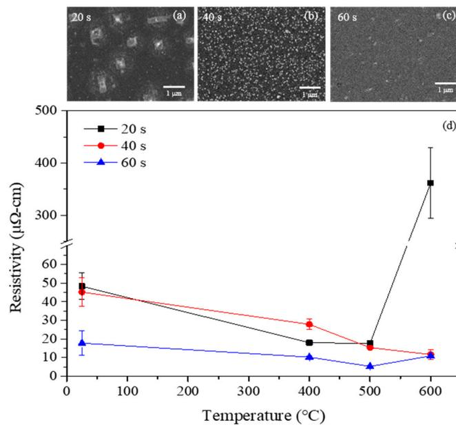
**Figure 7.** The surface morphologies of the 600 °C-annealed Cu(Mn) films deposited at the terminated OCP time of (a) 20 s, (b) 40 s, (c) 60 s, and (d) the electrical resistivity changes for the studied Cu(Mn) films annealed at an elevated temperature.
