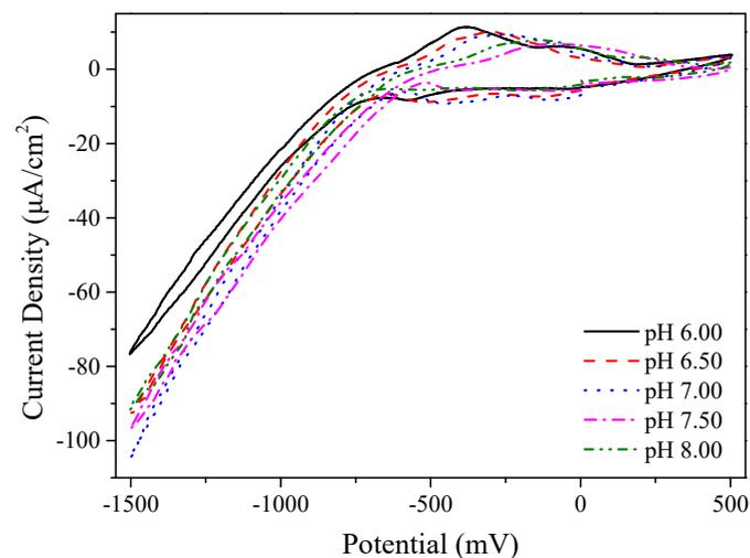
**Figure 1.** Cyclic voltammograms for the substrate in the Mn electrolyte with different pH values.
