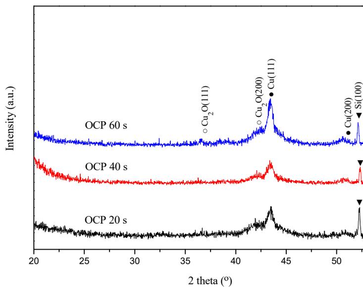
**Figure 6.** XRD results for the Cu(Mn) film deposited at the different terminated OCP times.
