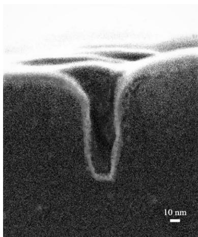
**Figure 9.** Cross-sectional SEM micrograph of Cu(Mn) film deposited in a via with an aspect ratio of 5 using 60 s terminated OCP time.
