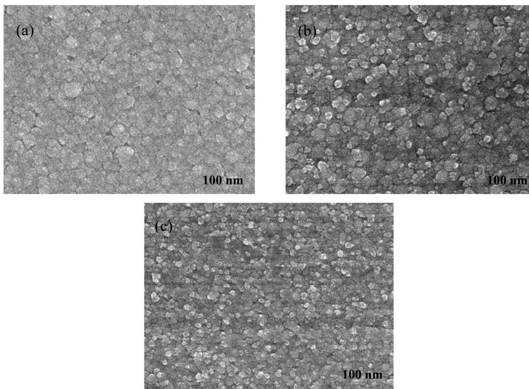
**Figure 5.** Surface morphologies of the Cu(Mn) films deposited in the Cu electrolytes, with various terminated OCP times of (a) 60 s, (b) 40 s, and (c) 20 s.
