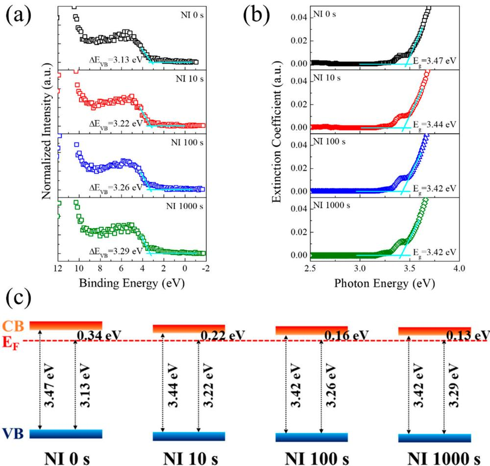
**Figure 4.** (a) Valence band offset ( $\Delta E_{VB}$ ) from valence band spectra; (b) optical band gap ( $E_g$ ) from extinction coefficient, and (c) the schematic energy band alignment of IGZO films as a function of the neutron irradiation time, including the relative energy position of Fermi level ( $E_F$ ) with respect to the conduction band minimum and the valence band maximum.
