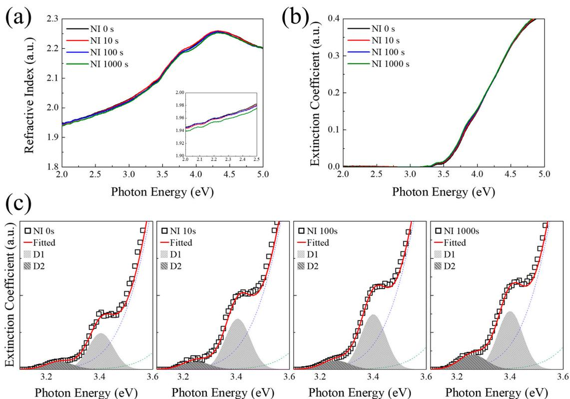
**Figure 3.** (a) Refractive index  $n$ ; (b) extinction coefficient  $k$  extracted using SE analysis, and (c) the evolution of the relative defect absorption areas below the conduction band of IGZO films for two distinct band edge states (D1 and D2), calculated by the deconvoluted Gaussian function fitting.
