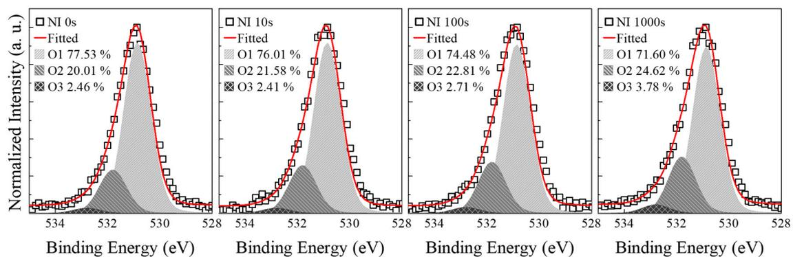
**Figure 2.** O 1s core level spectra deconvoluted with Gaussian fits as a function of the neutron irradiation time.
