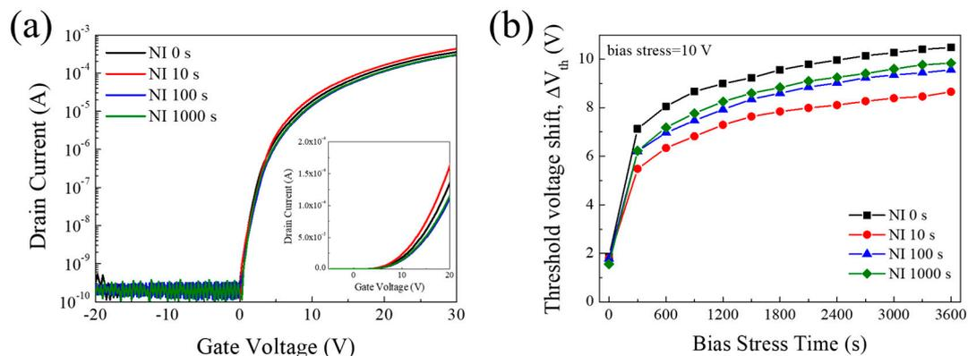
**Figure 5.** (a) Transfer curves (inset shows the linear scales) and (b) shift of threshold voltage under positive bias stress of IGZO TFTs as a function of the neutron irradiation time.
