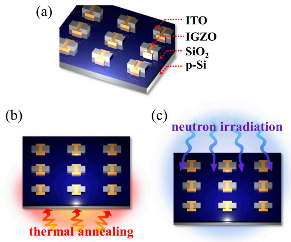
**Figure 1.** (a) Schematic illustration of the structure of IGZO TFTs; (b) conventional thermal annealing, and (c) the neutron irradiation process.
