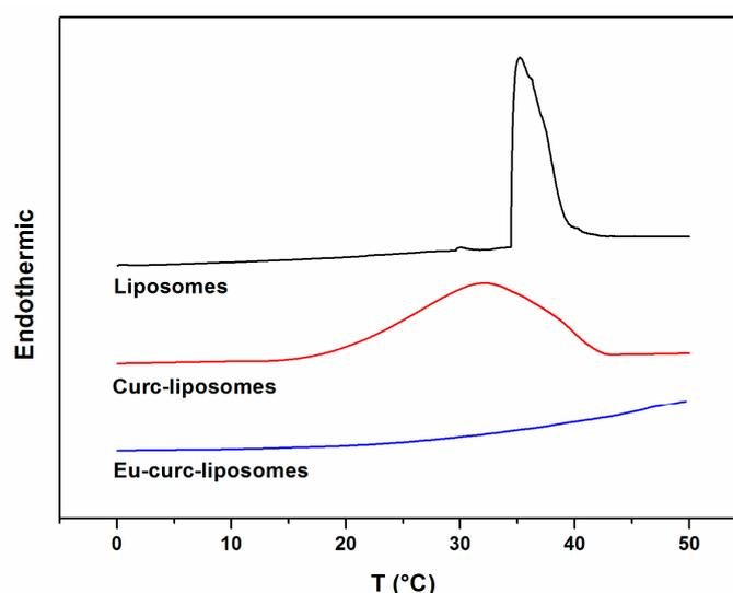
**Figure 3.** Differential scanning calorimetry (DSC) thermograms of liposomes, Curc-liposomes, and Eu-curc-liposomes.
