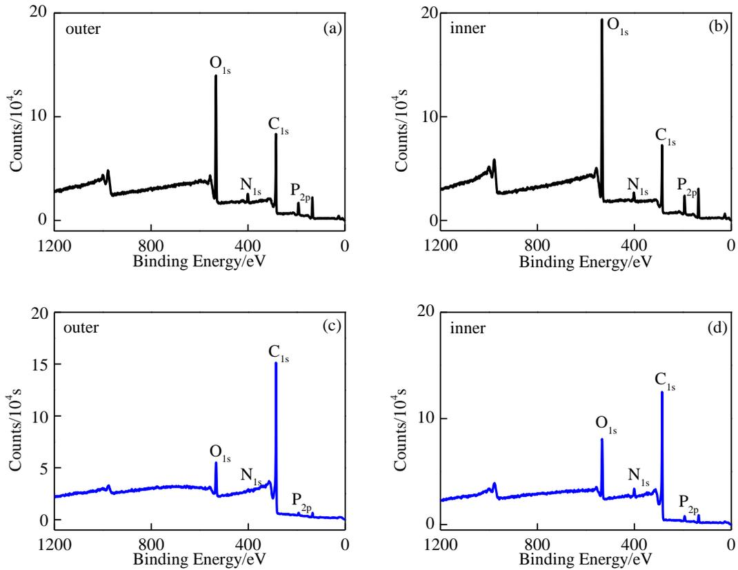
**Figure 2.** The composition of element for No.0 and No.3 outer and inner char layers.
