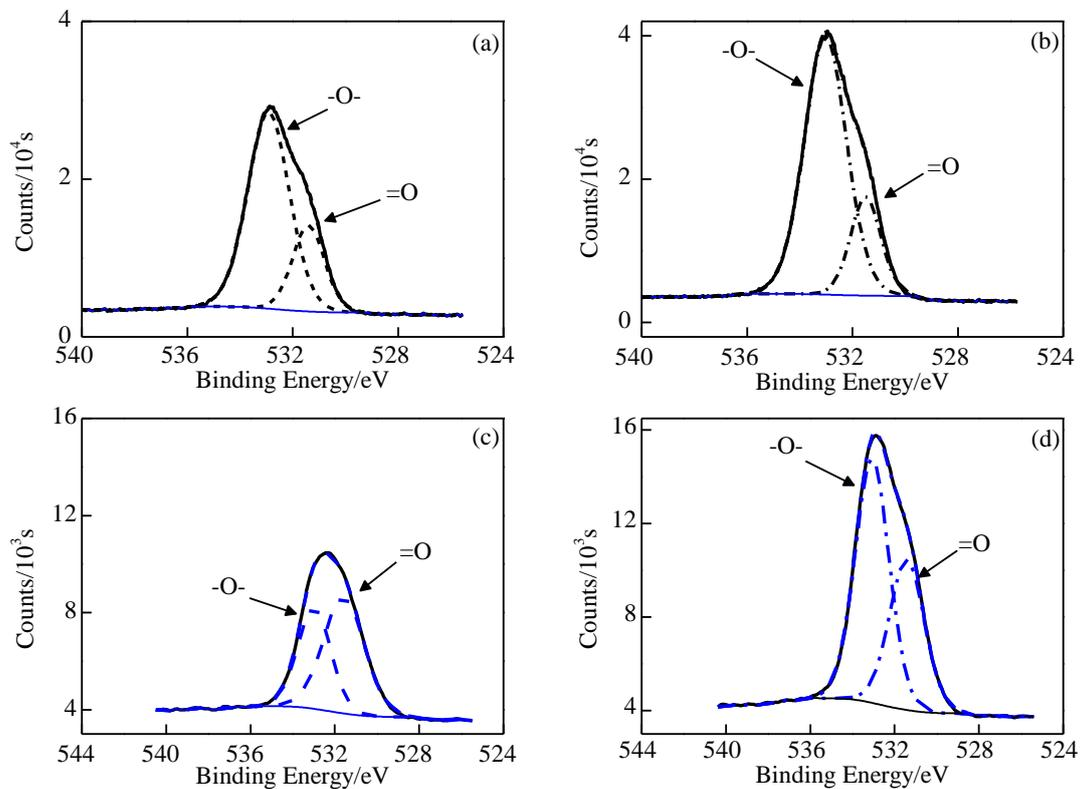
**Figure 3.** The O<sub>1s</sub> XPS spectrum: (a) outer No.0; (b) inner No.0; (c) outer No.3; and (d) inner No.3.
