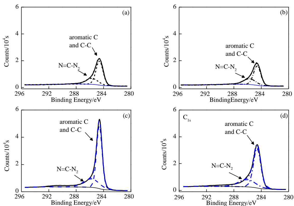
**Figure 5.** The C<sub>1s</sub> XPS spectrum: (a) outer No.0; (b) inner No.0; (c) outer No.3; and (d) inner No.3.
