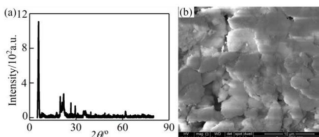
**Figure 1.** (a) The XRD pattern of MMT and (b) SEM image of MMT.
