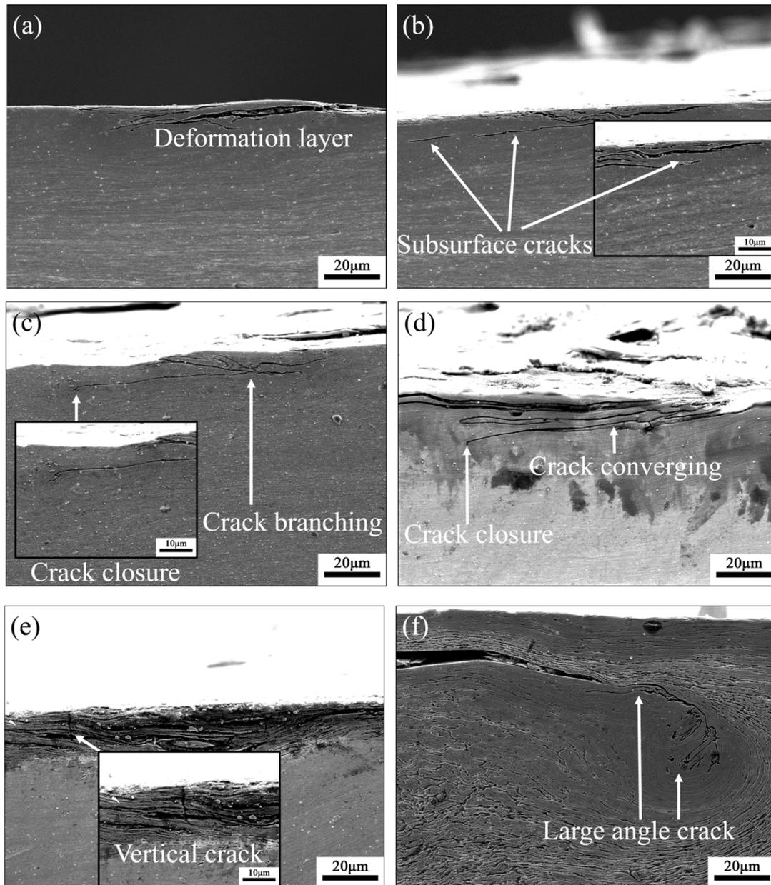
**Figure 8.** Micro-cracks in the cross-sections of the steels tempered at 550 °C after wear for different time, (a) 30 min, crack expanding inward; (b) 30 min, sub-surface crack expanding outwards; (c) 60 min, crack propagating; (d) 60 min, crack converging; (e) 120 min, vertical crack; (f) 120 min, sub-surface large-angle crack.
