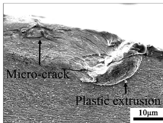
**Figure 6.** Cross-section morphology of the steel tempered at 680 °C after impact wear for 120 min.
