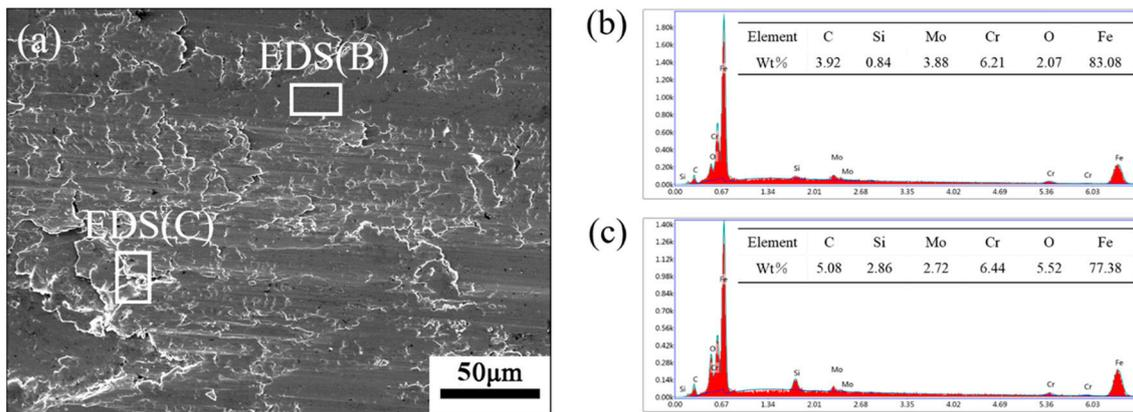
**Figure 4.** Surface wear morphology and EDS analysis of 680 °C tempered samples after 15 min wear. (a) Micro morphology of worn surface; (b) EDS analysis of region marked with EDS(B); (c) EDS analysis of region marked with EDS(C).
