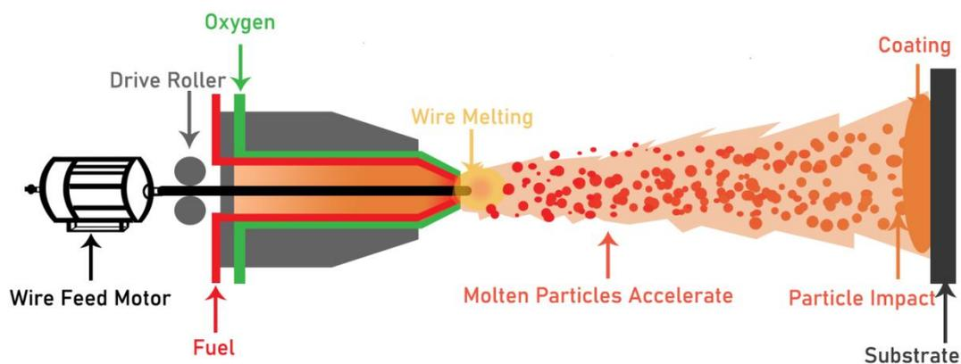
Figure 10. HAp coating using Flame Spray Technique.
