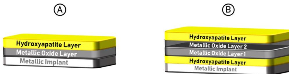
**Figure 11.** (A) Oxide layer in between metallic implant and HAp and (B) Bi-layer Metallic oxide coating.
