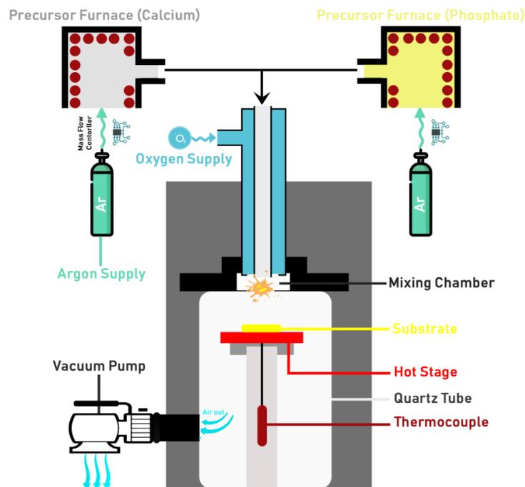
Figure 4. Schematic of HAp coating using Chemical Vapor Deposition (CVD).
