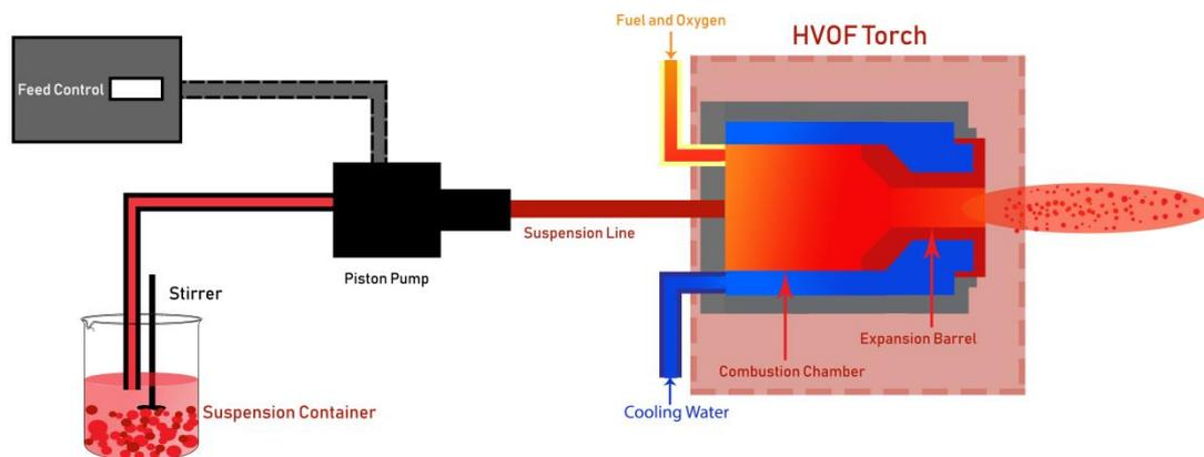
Figure 8. High velocity suspension flame spray (HVSFS).
