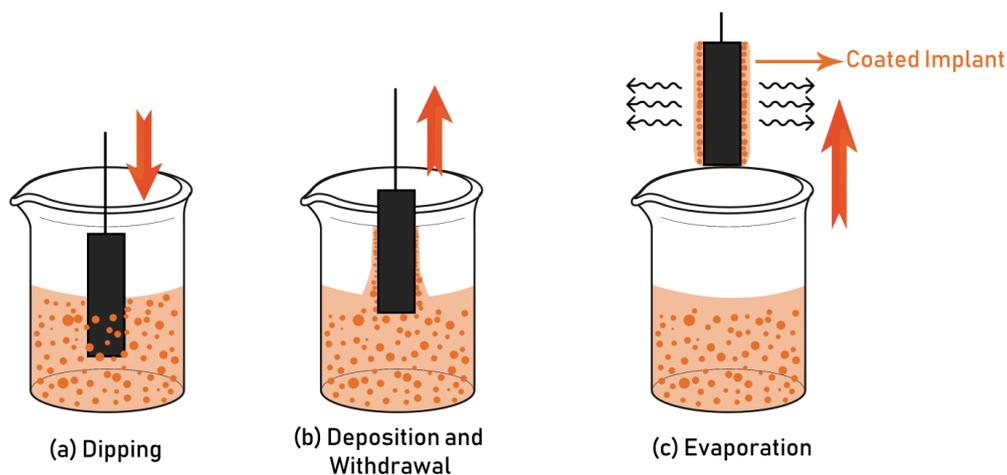
**Figure 2.** Schematic of Dip coating Process.
