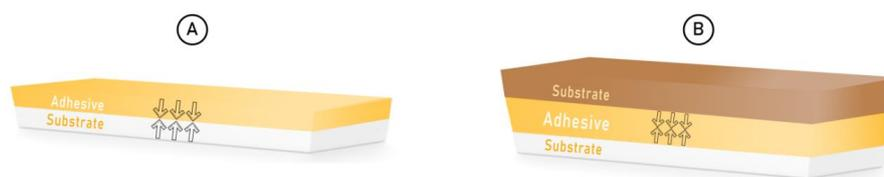
**Figure 1.** (A) adhesion and (B) cohesion forces between the adhesive layer and substrate [77].
