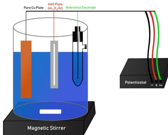
Figure 5. Schematic of Electro-chemical deposition Process.
