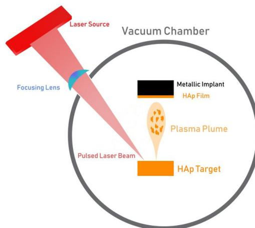
**Figure 9.** HAp coating using Pulsed Laser Deposition.
