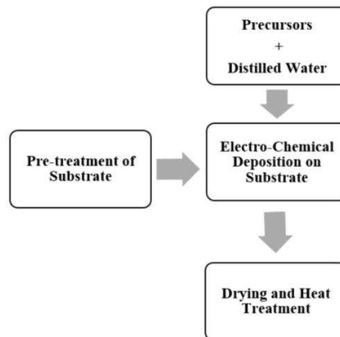
**Figure 6.** Block Diagram of Electro-Chemical Deposition Process.
