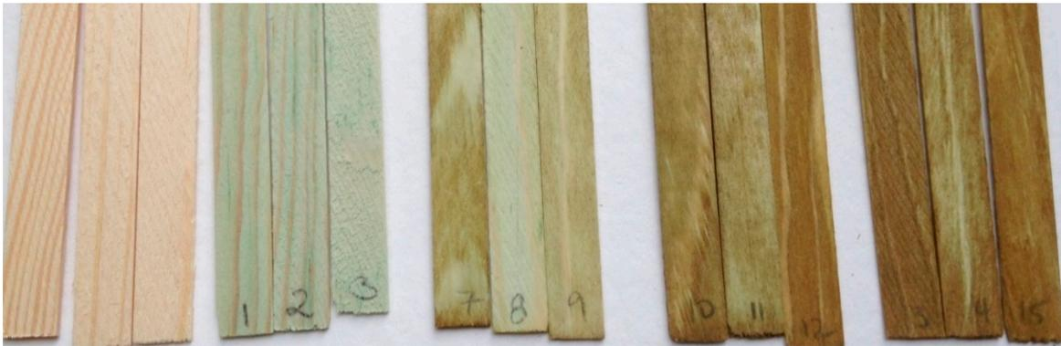
**Figure A1.** The effect of hydrogen peroxide concentration on the color of spruce treated with MBCC (left to right: untreated, MBCC treated (no peroxide), MBCC-treated 10% peroxide at pH 6, MBCC treated 20% peroxide at pH 5, 30% peroxide at pH 4).
