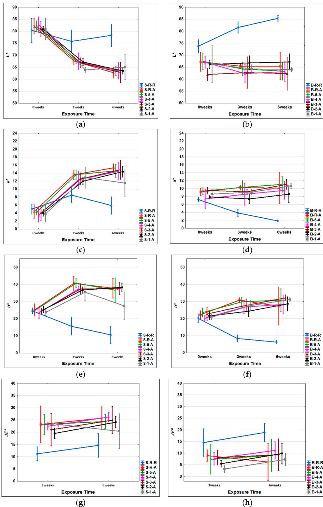
**Figure 3.** Colour changes in tested wooden surfaces during AW: (a)  $L^*$  changes on spruce; (b)  $L^*$  changes on beech; (c)  $a^*$  changes on spruce; (d)  $a^*$  changes on beech; (e)  $b^*$  changes on spruce; (f)  $b^*$  changes on beech; (g)  $\Delta E^*$  changes on spruce; (h)  $\Delta E^*$  changes on beech.
