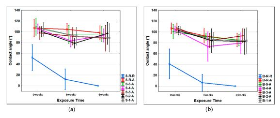
**Figure 5.** Water contact angle changes in tested wooden surfaces during AW: (**a**) Water contact angle (°) on tested spruce samples; (**b**) Water contact angle (°) on tested beech samples.
