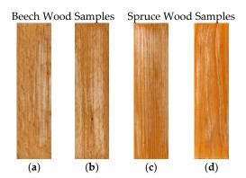
**Figure 2.** Oil-based coating after 6 weeks of AW. (**a**) Beech wood without pre-treatment (B-R-O); (**b**) beech wood with caffeine pre-treatment (B-5-O) achieved the best results from the tested oil-coated variants; (**c**) spruce wood without pre-treatment (S-R-O); (**d**) spruce wood with 10% FN-NANO<sup>®</sup> treatment achieved the best results from the tested oil-coated variants (S-1-O).
