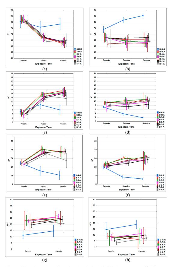
**Figure 3.** Colour changes in tested wooden surfaces during AW: (a)  $L^*$  changes on spruce; (b)  $L^*$  changes on beech; (c)  $a^*$  changes on spruce; (d)  $a^*$  changes on beech; (e)  $b^*$  changes on spruce; (f)  $b^*$  changes on beech; (g)  $\Delta E^*$  changes on spruce; (h)  $\Delta E^*$  changes on beech.
