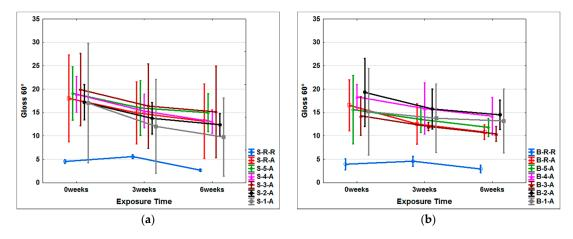
**Figure 4.** Gloss changes in tested wooden surfaces during AW: (**a**) Gloss changes on tested spruce samples; (**b**) Gloss changes on tested beech samples.
