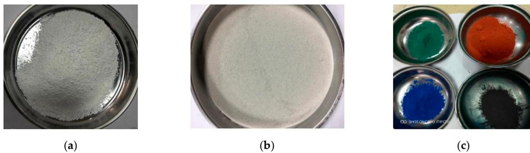
**Figure 4.** Functional fillers: (a) Titanium dioxide; (b) Floating beads; (c) Inorganic color pigments.
