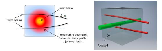
**Figure 3.** General scheme for the laser-induced deflection (LID) photothermal technique (**left**) and the measurement concept for rectangular substrate geometries (**right**).
