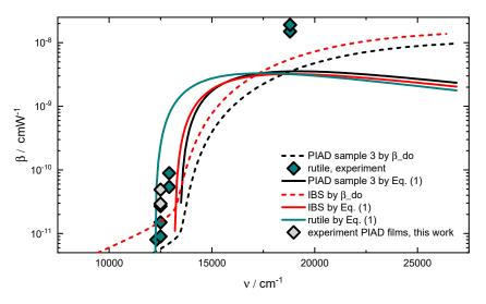
**Figure 9.** Measured TPA coefficients from rutile and PIAD  $TiO_2$  compared to simulations in terms of Equations (1), (3), and (4).
