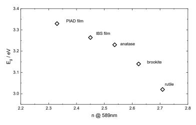
Figure 2. Correlation between optical gap and refractive index for the TiO<sub>2</sub> modifications from Table 1.
