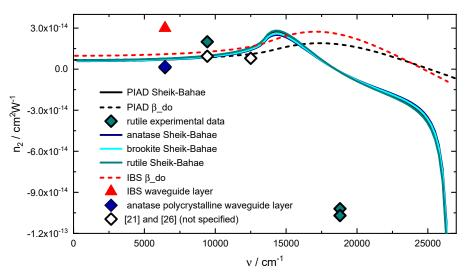
**Figure 10.** Measured nonlinear refractive indices from different TiO<sub>2</sub> modifications compared to simulations in terms of the Sheik–Bahae approach as well as Equations (3) and (4).
