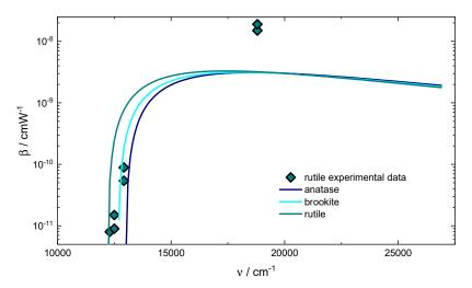
**Figure 1.** Two-photon absorption (TPA) coefficient as calculated from Equation (1) for crystalline TiO<sub>2</sub> modifications (solid lines; input data according to Table 1). Symbols: Experimental data reported in References [19,25] for rutile, as obtained from Z-scan techniques.
