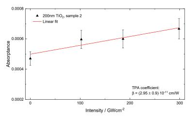
Figure 7. Absorptance versus laser intensity and the TPA coefficient for sample 2.
