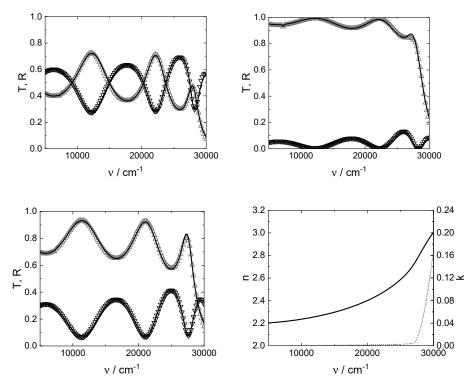
**Figure 5.** Modeled (solid line) and measured transmittance (up triangles) and reflectance (down triangles) at 60° for s- (**top left**) and p-polarizations (**top right**) and at near-normal incidence (**bottom left**) for sample 3 and modeled optical constants (**bottom right**, refractive index: Solid line, left axes; extinction coefficient: Dotted line, right axes).
