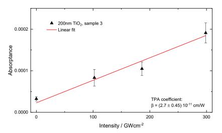
Figure 8. Absorptance versus laser intensity and the TPA coefficient for sample 3.
