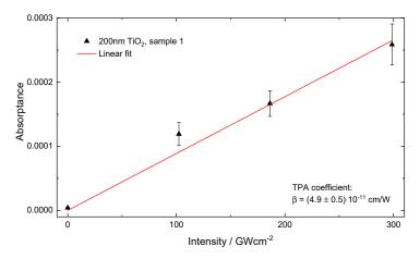
Figure 6. Absorptance versus laser intensity and the TPA coefficient for sample 1.
