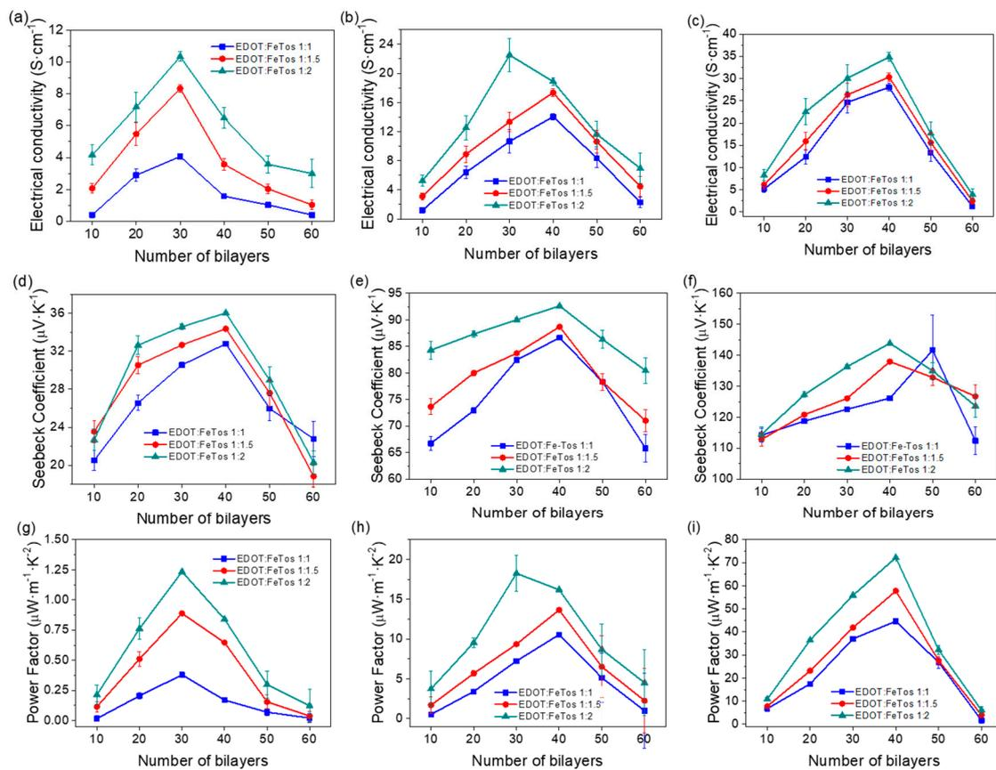
**Figure 7.** Electrical conductivity of (a) MWCNT–PEDOT nanoparticles, (b) DWCNT–PEDOT nanoparticles and (c) SWCNT–PEDOT nanoparticles. Seebeck coefficient of (d) MWCNT–PEDOT nanoparticles, (e) DWCNT–PEDOT nanoparticles and (f) SWCNT–PEDOT nanoparticles. Power Factor of (g) MWCNT–PEDOT nanoparticles, (h) DWCNT–PEDOT nanoparticles and (i) SWCNT–PEDOT nanoparticles as a function of the number of bilayers.
