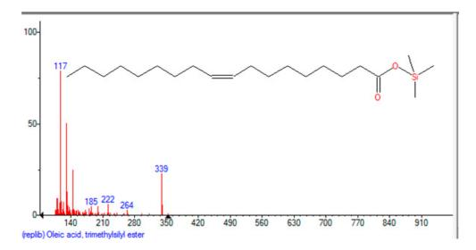
**Figure S31.** The EI mass spectrum of the GC peak corresponding to the alkenyl chain of **4** as identified from the NIST database (fragmentation pattern proposed as oleic acid trimethylsilyl acid).
