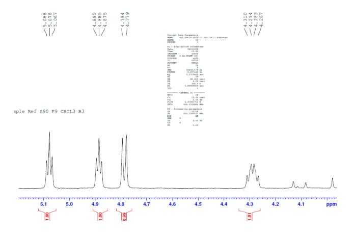
Figure S10 <sup>1</sup>H NMR spectrum of 2 in CDCl<sub>3</sub> (500 MHz)
