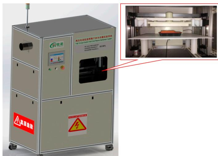
**Figure 1.** The schematic diagram of the high-voltage electric field cold plasma (HVCP) treatment for carrot juice.
