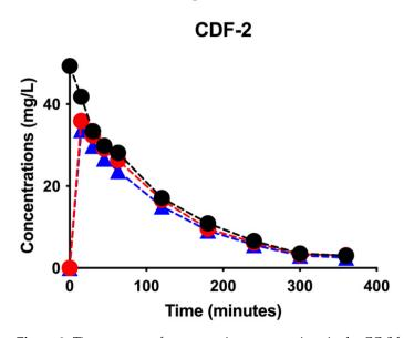
Figure 2 shows the time courses of vancomycin concentrations in the CC, inlet, outlet, and instantaneous effluent ports in the two sessions in the CD mode.
