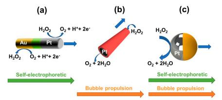
**Figure 2.** Catalytic micromotors for biosensing applications and related propulsion mechanisms. (a) Nanowires; (b) Tubular micromotors and (c) Janus micromotors.
