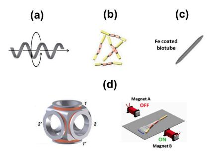
**Figure 3.** Magnetic micromotors for biosensing applications and related propulsion mechanisms. (a) Helical swimmers; (b) Flexible nanowires and (c) Microdraggers. Part (d) shows and schematic of the propulsion mechanisms based on Helmholtz coils (left part) or permanent magnets (right part). Reproduced with permission from ref. [53] (a,d), American Chemical Society; ref. [54] (b,d), Wiley and ref. [55] (c), Wiley.
