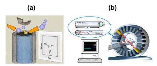
**Figure 5.** Transduction mechanisms for micromotors tracking in biosensing schemes. (**a**) Electrode impact voltammetry: schematic of a micromotor impacting a carbon microfiber electrode surface and the corresponding electrochemical signal generated. (**b**) Positron emission tomography. Reproduced with permission from ref. [61] (**a**), American Chemical Society and ref. [62] (**b**), American Chemical Society.
