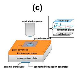
**Figure 4.** Ultrasound micromotors for biosensing applications and related propulsion mechanism. (a) Nanowires; (b) Iron-oxide loaded red blood cells (c) Schematic of the experimental set-up and propulsion mechanism. Reproduced with permission from ref. [32] (a), American Chemical Society; ref. [58] (b), American Chemical Society and [59] (c), American Chemical Society.
