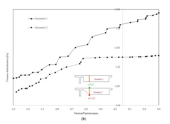
**Figure 10.** Pressure at specified cross section; the cross sections are determined to be: (**a**) at the beginning of the diverging section; and (**b**) at the immediate end of diverging section.
