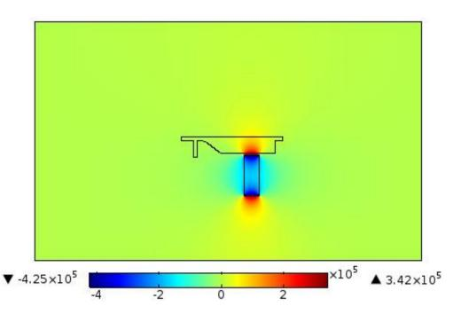
**Figure 12.** The magnetic distribution: the field maximum is located near the pole and there exists a rapid decay in the magnitude of magnetic field. The magnet only affects a small vicinity around it.
