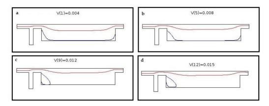
**Figure 6.** Change in streamlines by increasing velocity of auxiliary channel: (**a**) 4 mm/s; (**b**) 8 mm/s; (**c**) 12 mm/s; and (**d**) 15 mm/s. By increasing the velocity, the streamlines are lifted up and detached from the wall. A circulation zone will be formed above a threshold velocity.
