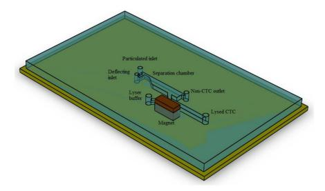
**Figure 1.** 3D schematic of the designed biochip composed of separator and mixer subunits; as can be observed, two units are arranged in serial configuration. In the first chamber, the CTCs are separated from the background cell by implementation of magnetic force and in the mixer unit by utilization of alternating voltage the mixing is achieved.
