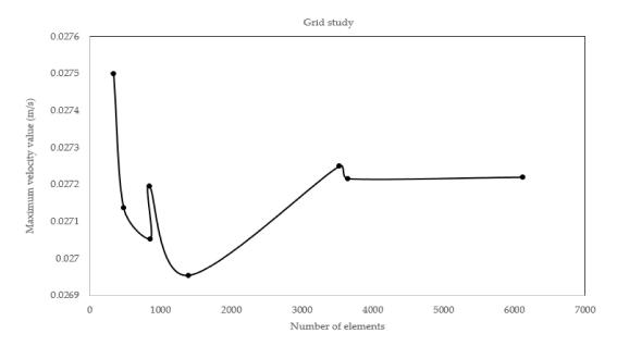
**Figure 8.** The way by which the domain is discretized has profound effect on accuracy of solution. Increasing number of elements increases both the accuracy and run time. The solution must be independent of element number. As can be observed, if the domain is discretized with more than 3000 elements, the maximum velocity becomes independent of number of elements.
