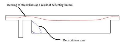
**Figure 5.** Consequences of adding ancillary channel: from the illustration, it is obvious that, by introducing this perpendicular flow, the streamlines are shifted upward. A circulation zone will also be formed at the bottom edge.
