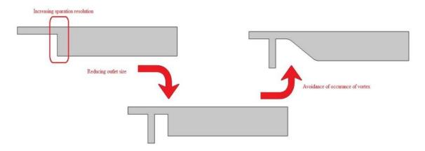
**Figure 4.** The evolution process of primary geometry: first by introducing an ancillary flow pf particles, dispersion is reduced and then, by gradual increase of cross-section, the induced vortices are avoided.
