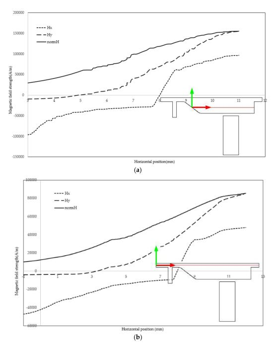
**Figure 14.** The magnetic field strength: (**a**) field magnitude in vicinity of bottom wall; and (**b**) field magnitude in vicinity of top wall.
