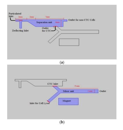
**Figure 2.** Top view of the geometry: (**a**) Section devised for isolating CTCs, composed of diverging section with 12 mm long in total composed of a 0.5 mm width inlet along with ancillary channel ending up to two distinct outlet one for tagged and one for non-tagged cells; and (**b**) Y-shaped section envisioned as mixing unit.
