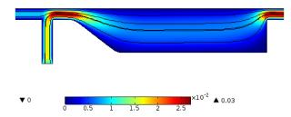
**Figure 11.** Velocity field within the separator geometry: at the cross section of two inlet flows, the velocity reaches its maximum. The streamlines are also illustrated. For applicability of device for extensive cellular study, one must ensure that the shear rate within the channel does not violate the maximum allowable shear. Otherwise, the cell viability is critically imperiled.
