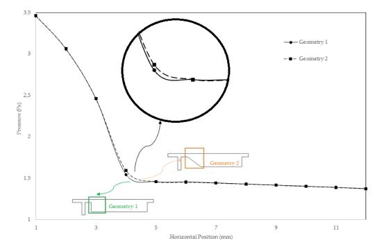
**Figure 9.** Pressure loss across the channel for two proposed geometry: in both geometries, the pressure decreases stream-wise and for Geometry 1 the loss is greater.
