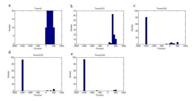
**Figure 16.** The histogram of particle vertical position at different times: the position is given in microns. As the time progressed (moving from graph (**a**–**e**)), the band width of particle distribution is reduced and the particles are all gathered in the same location.
