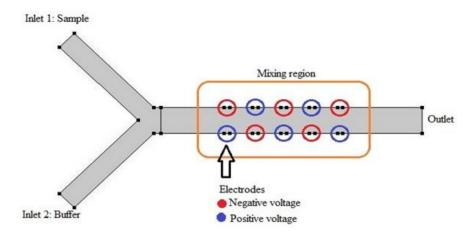
**Figure 3.** Mixer subunit; the main channel is 9 mm long and is 1 mm wide. As the flow passes the passage, it experiences alternating voltage executed by 10 electrodes which are positioned in zigzag configuration. The slip velocity plays a key role in mixing two parallel streams.
