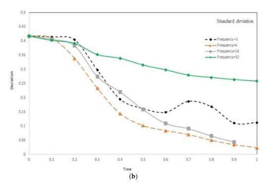
**Figure 19.** Assessing quality of mixing: (a) Deviation in pixel intensities at outlet versus time at different voltages: by increasing voltage the deviation is reduced. (b) Deviation in pixel intensities at outlet versus time at different frequencies: Mixing first improves as the frequency rises but above a certain frequency the performance deteriorates by further increase in frequency.
