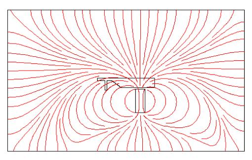
**Figure 13.** The magnetic field lines: the lines form an asymmetrical pattern with high density near the poles and low densities at other places.
