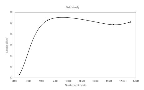
**Figure 18.** The accuracy of numerical solution is tightly bound to the grid. Increasing number of element increases both the accuracy and run time. The solution must be independent of element number. If the domain is discretized with more than 11,000 elements, the mixing index becomes independent of number of elements.
