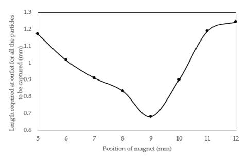
**Figure 15.** The position of magnet versus the required size of outlet: as the magnet moves in horizontal position far away from inlet particle, dispersion decreases and reaches a minimum value above this extreme point further moving of magnet increases the distance between particles hitting the bottom wall.
