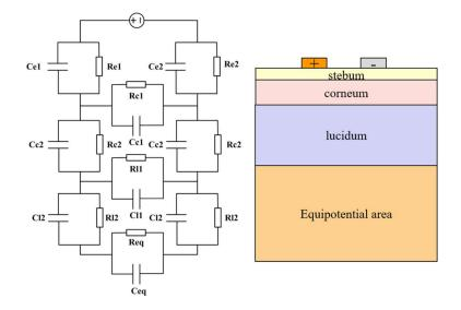
**Figure 4.** Equivalent circuit of human skin impedance measurement, which considers the layered nature of the skin, so the layered impedance was built vertically as well as the interlayer skin impedance in the horizontal direction [40].
