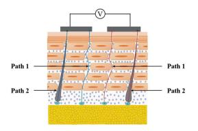
**Figure 2.** Schematic of the two transport paths for ions in dermis. Path 1 represents ions moving along the dermis–viable epidermis–SC through the intercellular lipid bilayer path; path 2 represents ion transport directly through the sweat glands to the skin surface.
