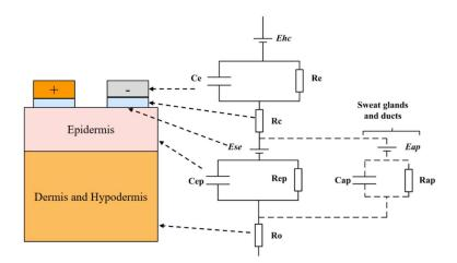
**Figure 5.** Equivalent circuit of human skin impedance measurement, which stressed the layered structure and the skin appendages [12].
