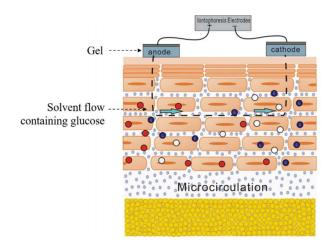
**Figure 7.** Schematic illustration of the principle of reverse iontophoresis showing an iontophoresis extraction device supplying a constant current to an anode and cathode.
