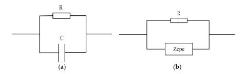
**Figure 3.** Two simple impedance models: (a) represents the initial RC skin impedance model; (b) represents the improved model based on (a) and considers the biological characteristics of the skin; the capacitance element was replaced by the constant phase angle element.
