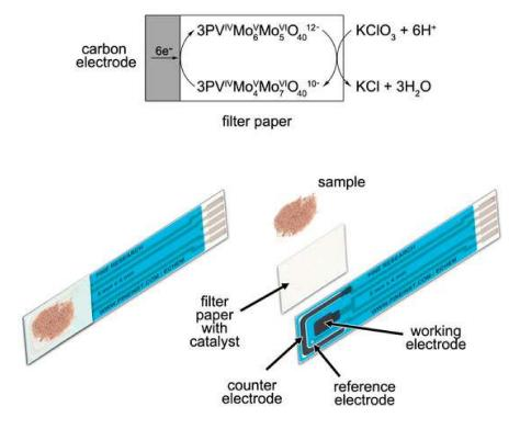
**Figure 6.** Paper-based electrochemical detection of chlorate. (Reproduced from Ref. [131], an open-access article distributed under the terms and conditions of the Creative Commons Attribution (CC BY) license (http://creativecommons.org/licenses/by/4.0/)).
