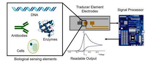
**Figure 1.** Scheme of an electrochemical biosensor. Biological sensing elements are coupled to electrodes. These traduce the signal to deliver a readable output.
