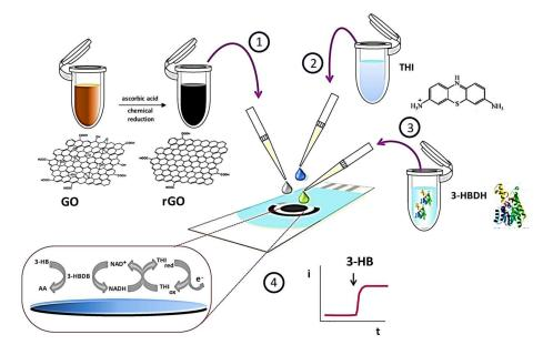
**Figure 5.** Scheme of the steps involved in the preparation and functioning of the 3-hydroxybutyrate dehydrogenase (3-HBDH)/thionine (THI)/reduced graphene oxide (rGO)/screen-printed carbon electrode (SPCE) biosensor. (Reproduced from Ref. [37], an open-access article distributed under the terms and conditions of the Creative Commons Attribution (CC BY) license (http://creativecommons.org/licenses/by/4.0/)).
