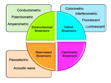
Figure 2. Four different classes and sub-classes of biosensors based on the type of transducer.
