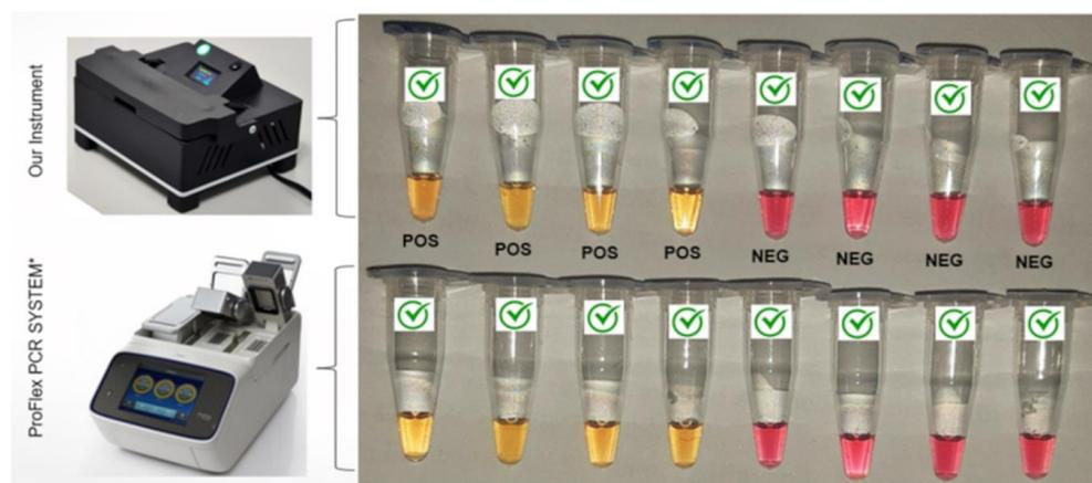
**Figure 7.** Comparison of RT-LAMP colorimetric reactions performed in a conventional Applied Biosystems ProFlex PCR System thermocycler (used in the LAMP mode) and our instrument. Yellow reactions are considered positive, and pink reactions are negative.
