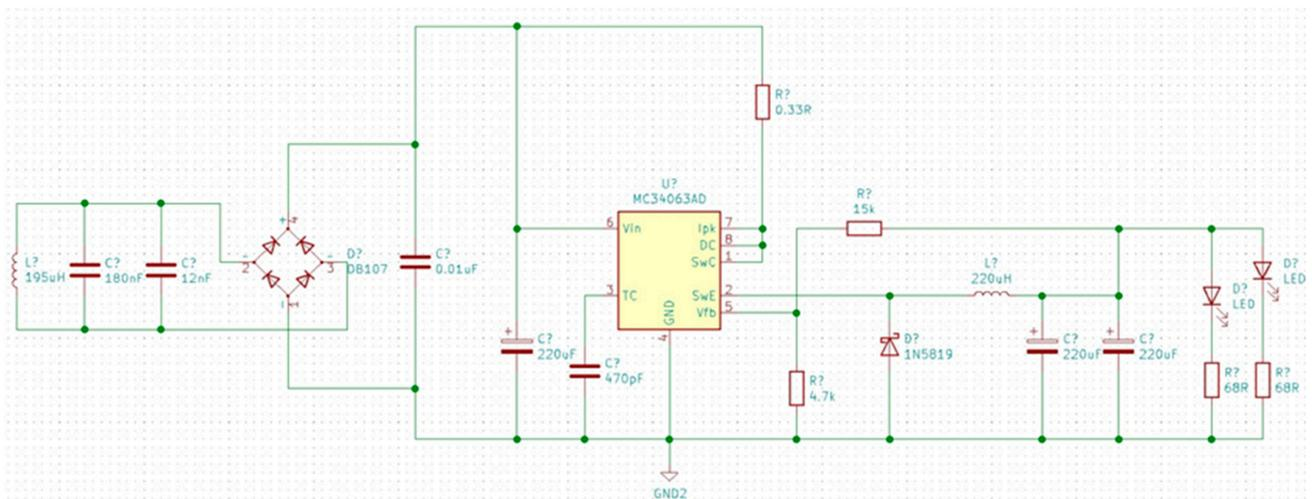
Figure 9. Electrical diagram of receiver module.
