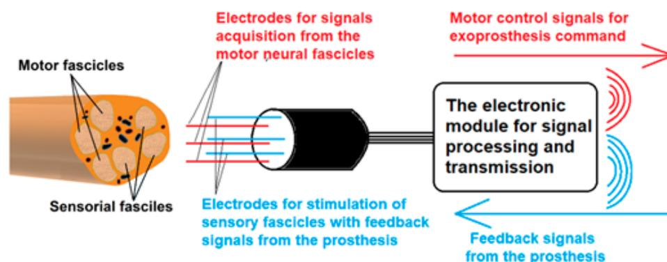
**Figure 1.** Conceptual design of the developed system, which provides a bidirectional connection with the wirelessly connected prosthesis.
