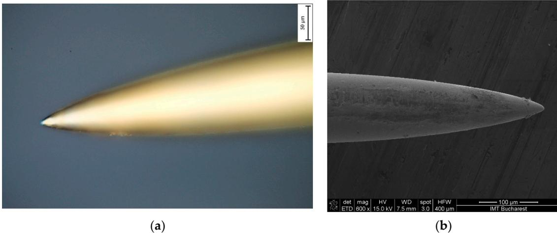
**Figure 6.** (a) Optical image (Leica microscope 50×-BF) of the needle used in our experiments; (b) SEM image (Nova™ NanoSEM 630) of the needle used for our plug electrode system.
