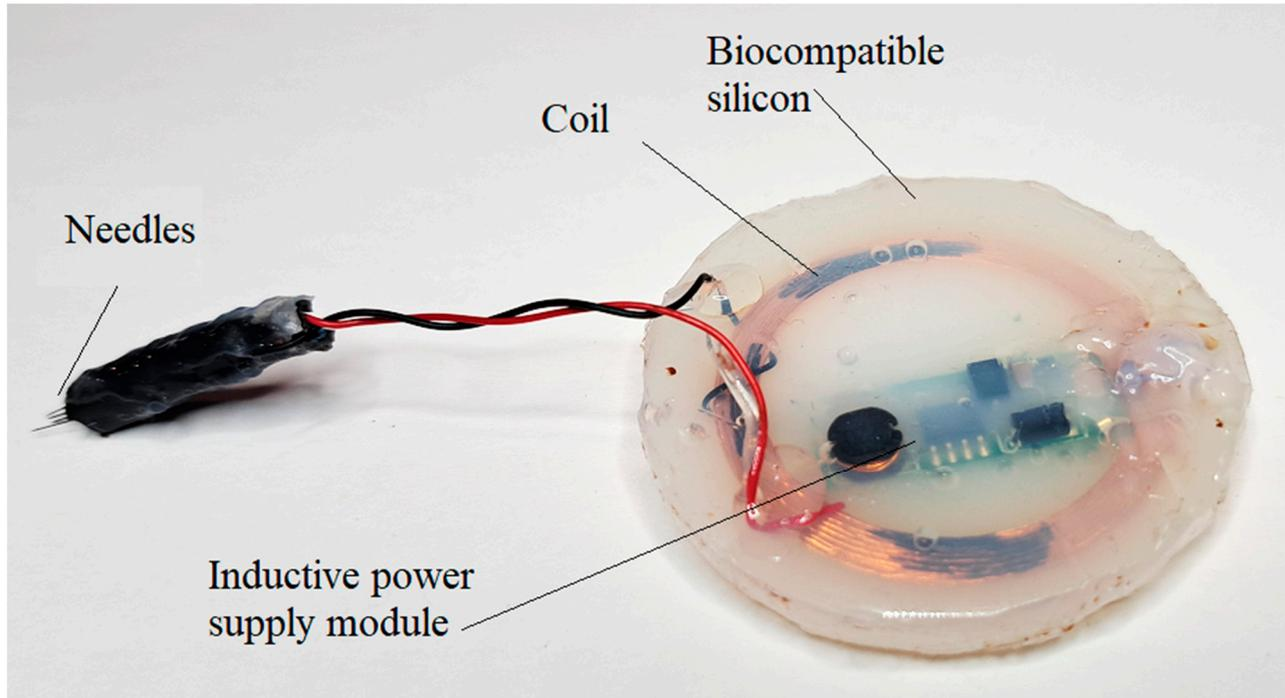
**Figure 11.** The module equipped with plug electrode designed to send signals to the neuronal fascicle.
