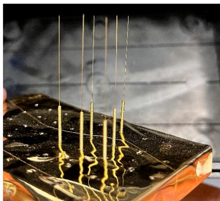
**Figure 5.** Layout of the needle support used for metal deposition.
