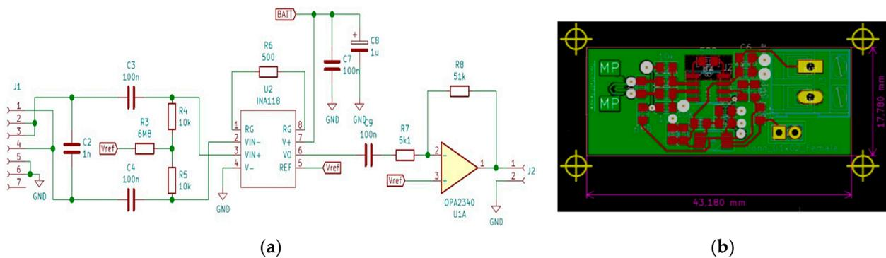
**Figure 7.** (a) The circuit diagram of the front-end module and (b) the front-end PCB.
