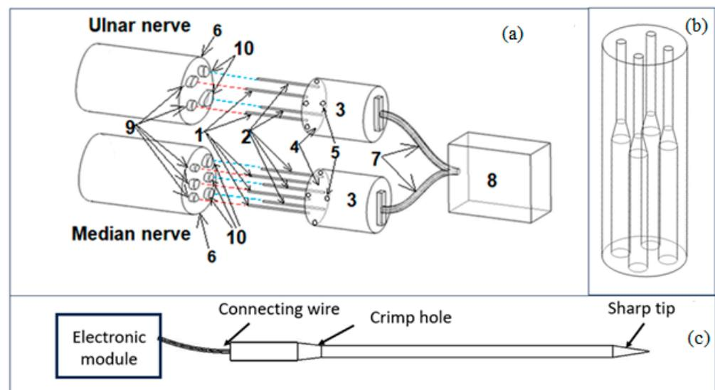
**Figure 3.** (a) Detailed schematic representation of the plug electrodes. (b) The support for fixing the needles. (c) The components of the needle-type electrodes.
