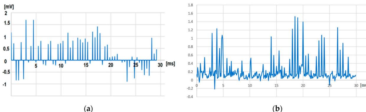
**Figure 15.** (a) Signals acquired with implanted module equipped with plug electrodes. (b) Signals acquired with implanted module equipped with cuff electrodes.
