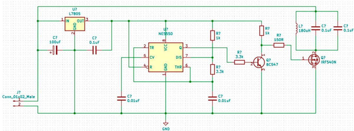
Figure 8. Electrical diagram of generator module.
