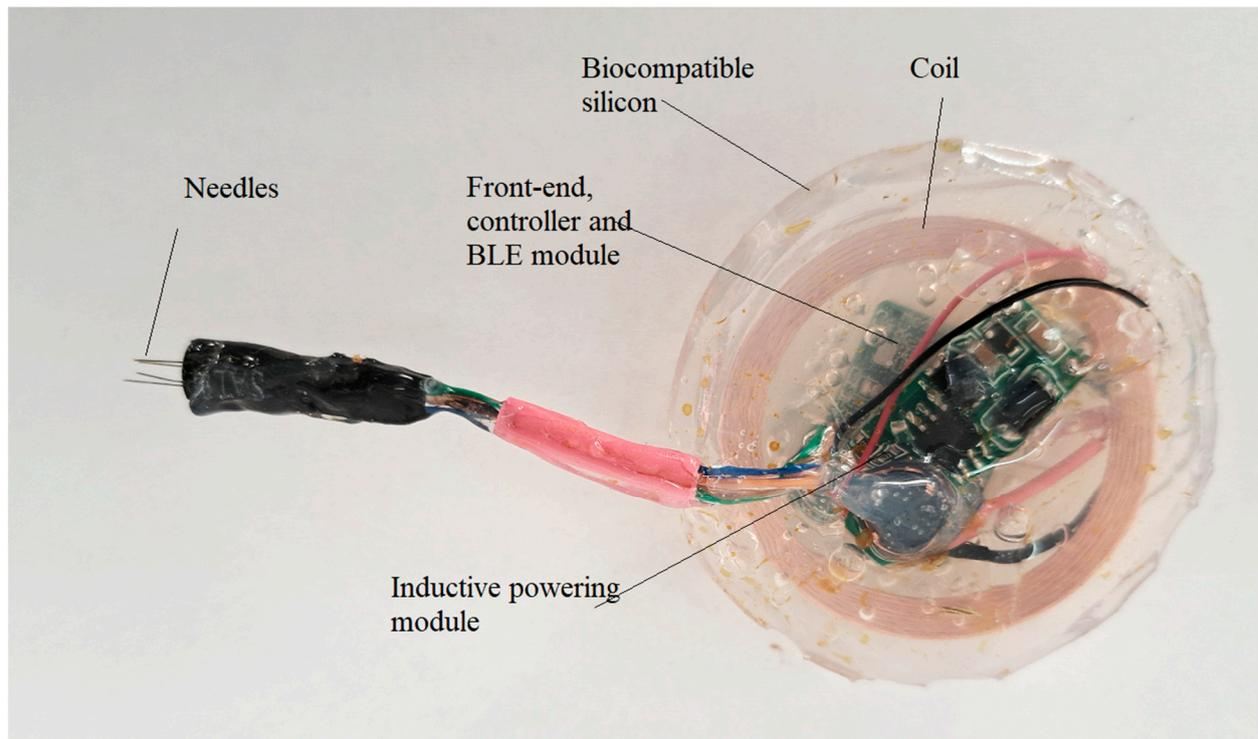
**Figure 10.** The module equipped with plug electrode designed to harvest signals from the neuronal fascicle.
