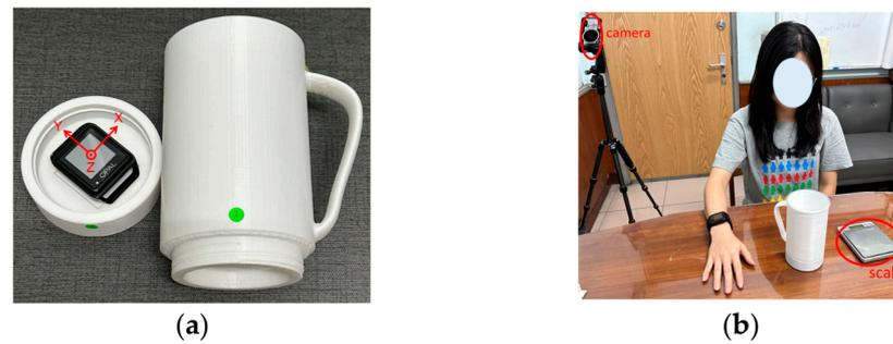
**Figure 1.** (a) The 3D-printed cup and the orientation of the OPAL sensor. (b) The experimental environment setting includes the wrist-worn sensor, a 3D-printed cup, a scale, and a synchronized camera.
