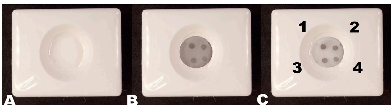
**Figure 2.** Vertical flow assay procedure. (A) Addition of the analyzed sample; (B) addition of CNP@MAb; (C) addition of 200  $\mu$ L washing buffer. Spike protein concentration: (1) 0.5 mg/mL; (2) 0.25 mg/mL; (3) 0.125 mg/mL; (4) 0.0625 mg/mL.
