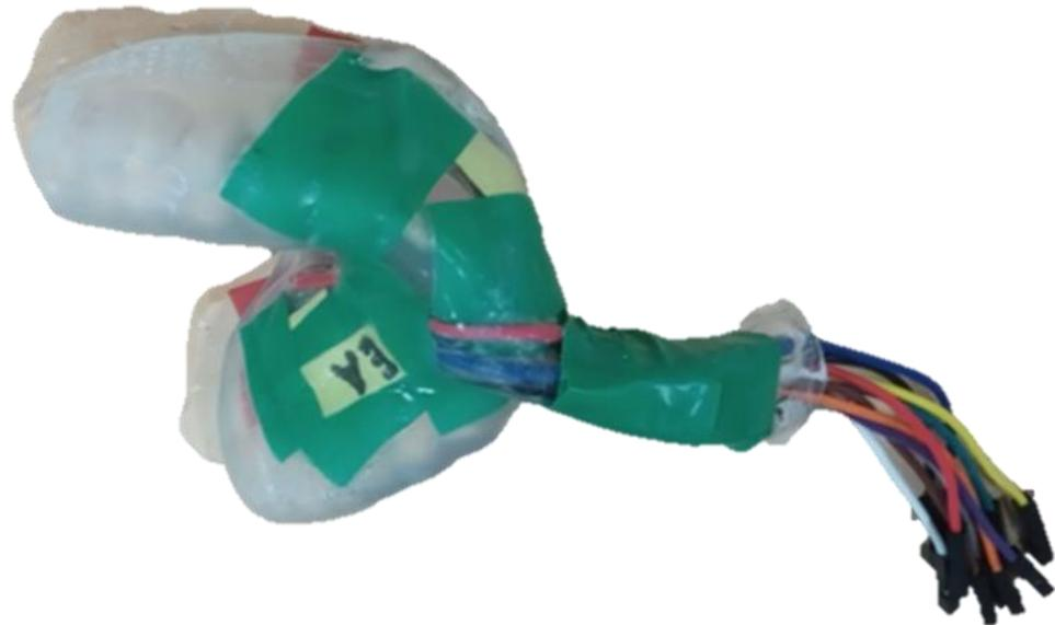
**Figure 2.** An EVA-encased mouthguard was situated on top of the cast with two MAX30102 sensors embedded. A cable was used to connect it to the MAX30102ACCEVKIT Evaluation System. Green electric tape was used to keep the wires in place during the forming process, while a yellow pH-sensitive comparator paper strip was positioned along the wires to detect potential water ingress.
