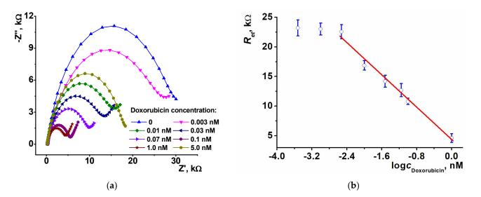
**Figure 7.** (a) The Nyquist diagrams obtained with GCE covered with polyPhTz (2.5 cycles) in the presence of TC-*alt* and DNA (20 min incubation, 1 mg/mL of DNA from salmon testes) after incubation in increasing concentrations of doxorubicin (20 min. incubation; (b) calibration graph of doxorubicin determination in semilogarithmic plots, average  $\pm$  S.D. for three individual sensors.
