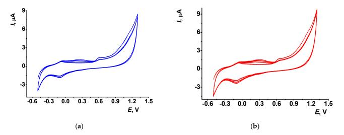
**Figure 1.** Cyclic voltammograms of PhTz polymerization recorded in phosphate buffer–acetone mixture (1:1 v/v) in the presence of 0.072 mM PhTz, scan rate 100 mV/s: (**a**) 2.5; (**b**) 3.5 cycles of potential.
