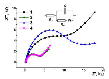
**Figure 5.** The Nyquist diagrams obtained with GCE covered with polyPhTz (2.5 cycles) in the presence of TC-*cone*, reagent ratio TC-*cone*: PhTz (mol/mol) = 0 (1), 1:4 (2), 1:2 (3) and 1:1 (4). Inset: equivalent circuit,  $R_s$ —solvent resistance,  $R_{et}$ —electron transfer resistance, W—Warburg impedance, Q—constant phaser element.
