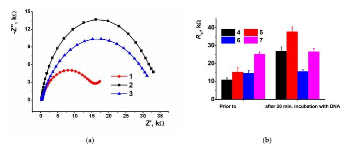
**Figure 6.** (a) The Nyquist diagrams obtained with GCE covered with polyPhTz (2.5 cycles) in the presence of TC-*cone* (1), TC-*paco* (2) and TC-alt (3) and coated with DNA (20 min incubation, 1 mg/mL of DNA from fish sperm); (b) comparison of the electron transfer resistance for various coatings of the GCE/PolyPhTz/DNA sensors prior to and after DNA loading: polyPhTz (4), poly-PhTz TC-*alt* (5), polyPhTz—TC-*cone* (6), polyPhTz—TC-*paco* (7).
