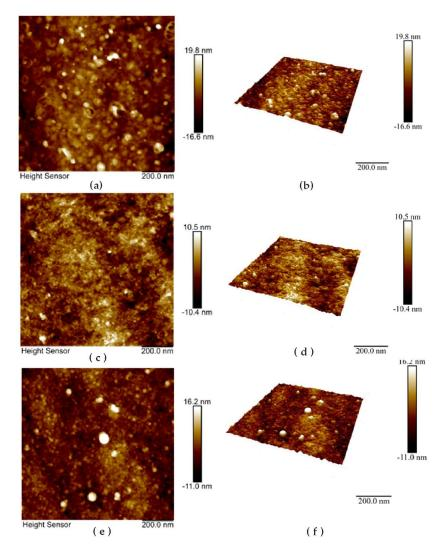
**Figure 3.** Morphology (**a**,**c**,**e**) and 3D models of the GCE surface (**b**,**d**,**f**) after electrodeposition of polyPhTz (**a**,**b**); polyPhTz in the presence of TC-*cone* (**c**,**d**); and that after 20 min exposition of 1 mg/mL DNA (**e**,**f**).
