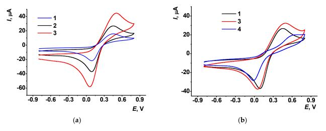
**Figure 2.** Cyclic voltammograms recorded in 0.01 M  $[Fe(CN)_6]^{3-/4-}$  solution on GCE (**a**), bare (1) and that covered with the polyPhTz synthesized in 2.5 (2) and 3.5 (3) potential cycles; (**b**) polyPhTz synthesized in the presence of TC*-cone* (3) and that after 20 min incubation of DNA (4) (2.5 cycles).
