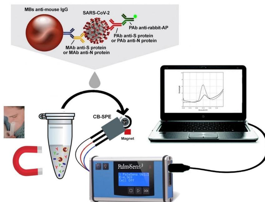
**Figure 12.** The MBs-based assay for SARS-CoV-2 detection in untreated saliva. Reprinted with permission from Elsevier from Ref. [152].
