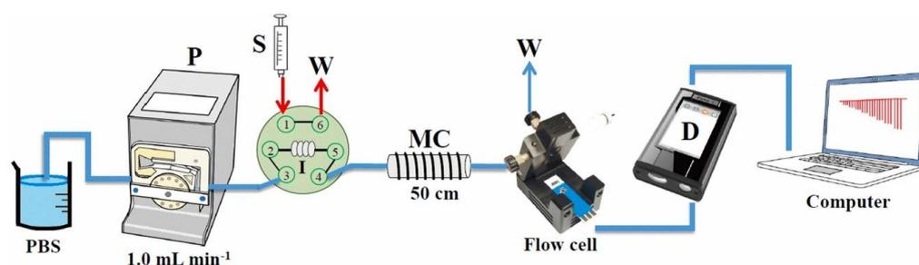
**Figure 11.** Illustration of FI-Amp system for uric acid determination using a CB-GO modified SPCE (PBS = 10 mM phosphate buffer pH 6.0, P = peristaltic pump, S = standard/sample, I = injection valve (150  $\mu\text{L}$ ), MC = mixing coil, W = waste, D = AC impedance electrochemical analyzer-simulator. Reprinted with permission from Elsevier from Ref. [149].
