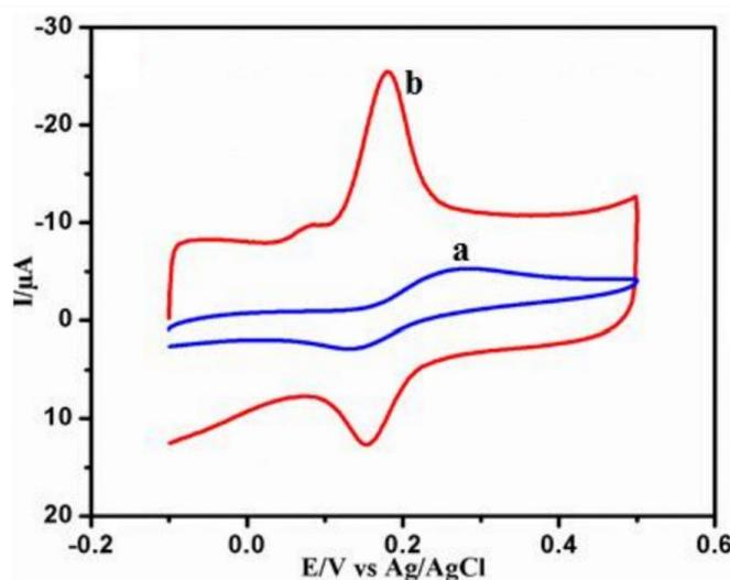
**Figure 5.** Cyclic voltammetry of bare SPCE (a) and f-MWCNT/SPCE (b) in the presence of  $500 \mu\text{mol L}^{-1}$  CT in  $0.05 \text{ mol L}^{-1}$  PB solution (pH 7.0) at a scan rate of  $50 \text{ mV s}^{-1}$ . Reprinted with permission from ESG from Ref. [113].
