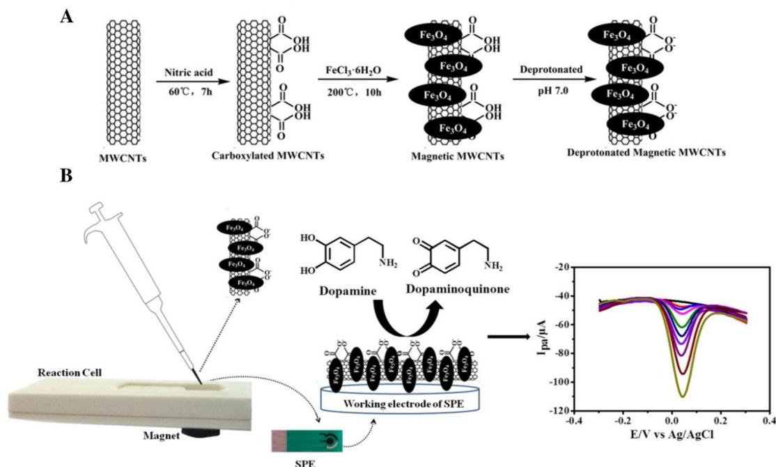
**Figure 6.** (A) Synthetic route of mMWCNTs. (B) Magnetism-assisted modification of SPE with mMWCNTs and electrochemical response of dopamine on mMWCNTs/SPE. Reprinted with permission from Elsevier from Ref. [121].
