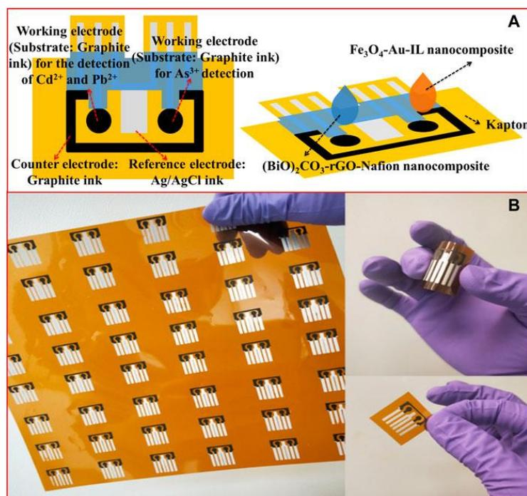
**Figure 2.** (A) Schematic diagram of the SPE. (B) Optical images of the SPE. Reprinted with permission from Frontiers from Ref. [27]. Subtitles: IL: L-cysteine.
