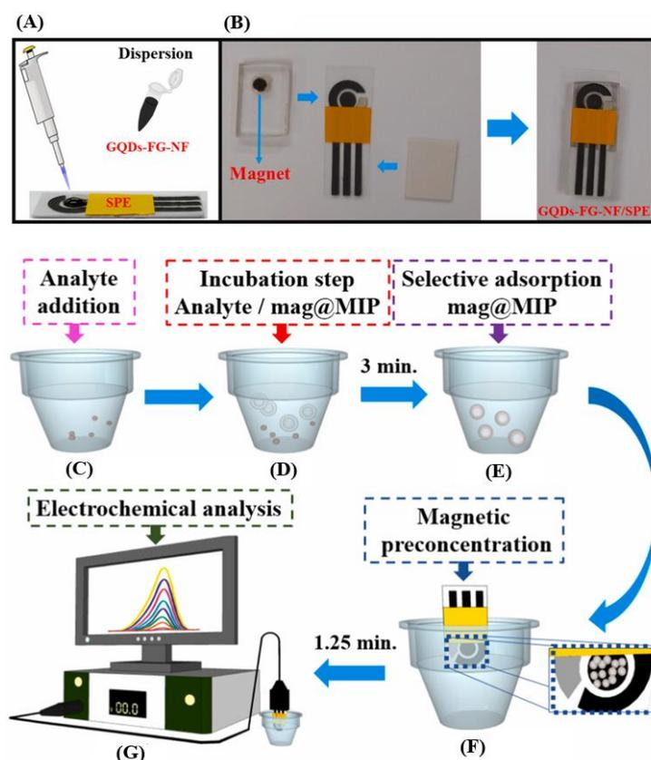
**Figure 13.** (A) SPE modification with GQDs-FG-NF and (B) fixing the magnet to the modified SPE. Sensor mechanism: (C) addition of the analyte; (D) incubation step with the mag@MIP in the analyte solution; (E) analyte adsorption by the mag@MIP; (F) separation of the analyte-mag@MIP with the electrode magnet (GQDs-FG-NF/SPE), and (G) steps of electrochemical analysis. Reprinted with permission from Elsevier from Ref. [156].
