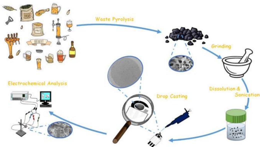
**Figure 14.** Biochar/SPE preparation scheme. Reprinted with the permission of Elsevier from Ref. [176].
