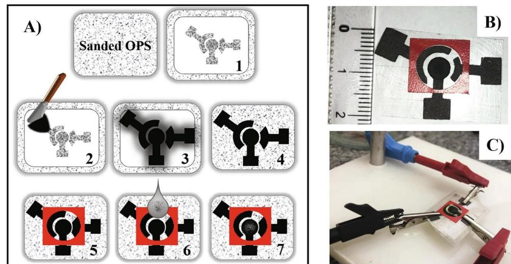
**Figure 9.** (A) Schematic representation of SPE preparation and modification. (B) Image of the final device. (C) Image of the final SPE connected to the potentiostat. Reprinted with permission from Elsevier from Ref. [124].
