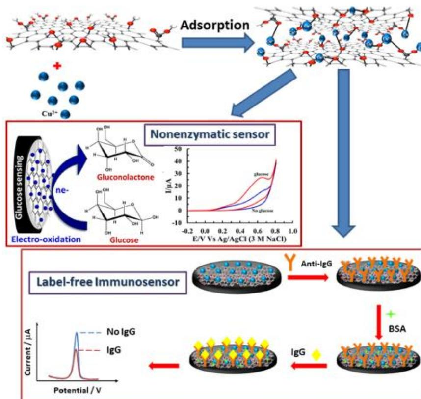
**Figure 3.** Fabrications of IgG immunosensor and non-enzymatic glucose sensor based on a versatile Cu(II)/GO-modified SPCE. Reprinted with permission from Frontiers from Ref. [44].
