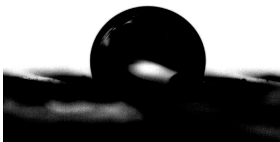
Figure S3. Surface contact angle ( 110^\circ ) of the PDMS micro-well array chip before plasma treatment determined using the contact angle measurement instrument (OCA 25, Dataphysics, Germany).
