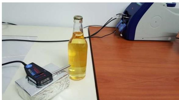
**Figure 3.** Portable Raman setup for the in-line analysis of drinks and spirits. A bottle of beer is placed as the sample.
