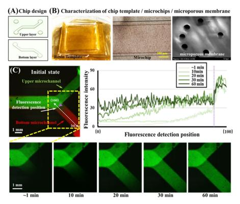
**Figure 2.** (**A**) Design of the 3D printed chip template. (**B**) Microscopy or SEM images of chip templates, microchips, and microporous membranes. (**C**) Fluorescence images and plots of fluorescence intensity profiles for the characterization of small molecule diffusion in a microchip. Green, RH-123 aqueous solution. Red, RH-B aqueous solution. Scale bar = 1 mm.
