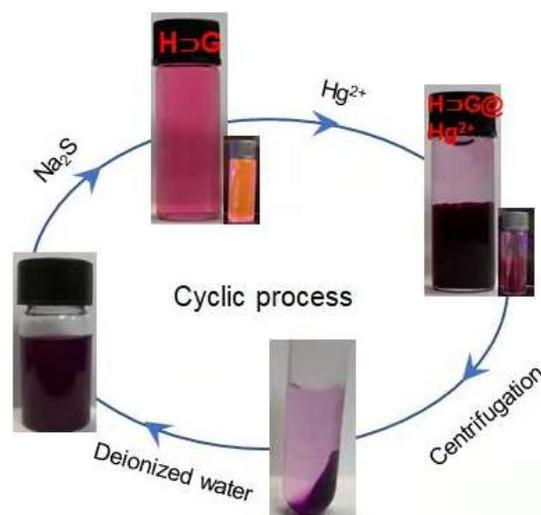
**Figure 8.** Representative photos during the process of sensing and removal of Hg<sup>2+</sup> and regeneration of absorbent material (H⊃G).
