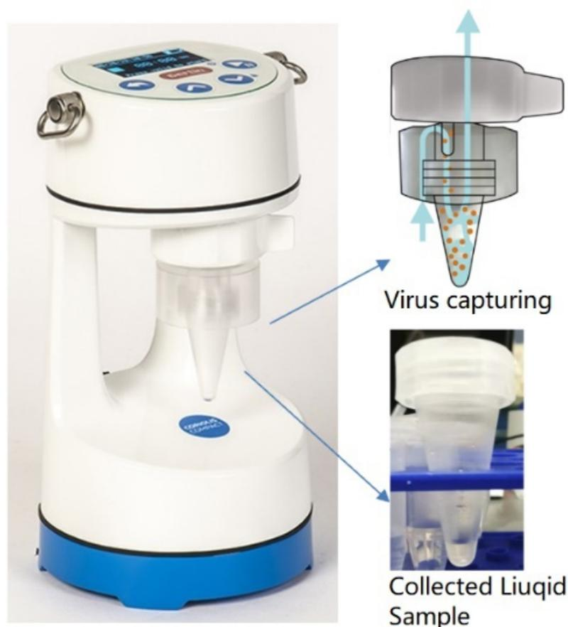
**Figure 5.** Coriolis Sampler used for capturing SARS-CoV-2 virus. Liquid samples containing SARS-CoV-2 virions were collected and centrifuged in a cone-shaped vial.
