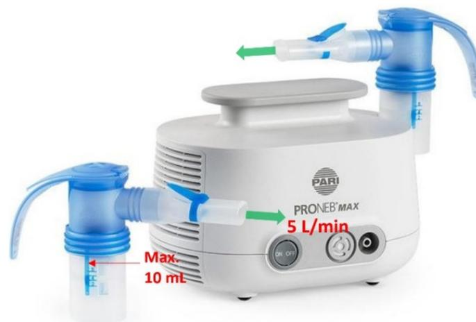
**Figure 3.** PRONEB nebulizer used to generate aerosols with heat inactivated SARS-CoV-2 virions in the test rig.
