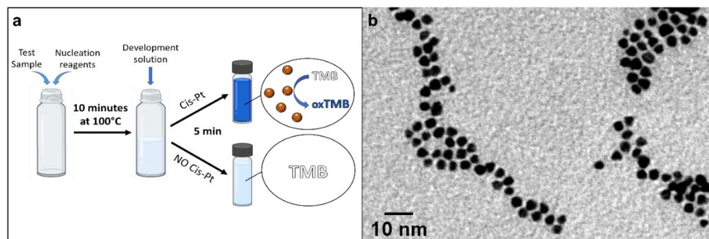
**Figure 1.** (a) Scheme of the two-step colorimetric method for the detection of cisplatin. In the presence of the chemotherapeutic drug, the reducing agent quickly promotes the formation of small (ca. 4 nm diameter) monodisperse PtNPs, which in turn catalyze the oxidation of the TMB chromogen, with consequent formation of a visible blue color. In the absence of cisplatin contaminations, the solution remains transparent. (b) Representative TEM image of the PtNPs formed from cisplatin.
