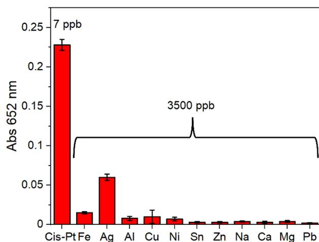
**Figure 3.** Selectivity of the colorimetric assay with respect to other toxic metal cations, in terms of absorbance signal measured after 5 min of reaction. Results are expressed as mean  $\pm$  SD of tripled experiments.
