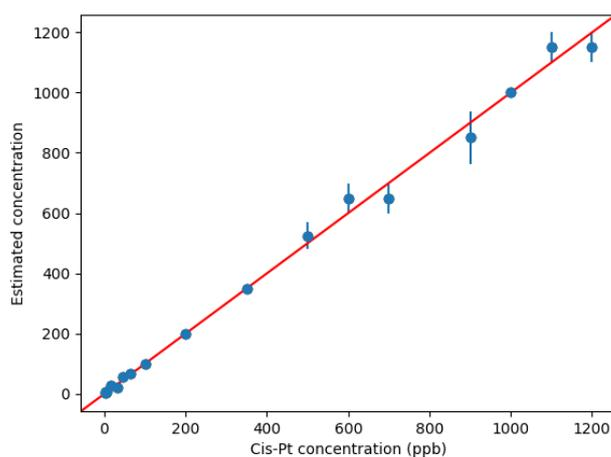
**Figure 5.** Quantitative measurements by ML: on the  $y$ -axis, the values predicted by the ML method are shown against the experimental concentrations of cisplatin (on the  $x$ -axis). For each concentration, the average value of the prediction is displayed by using a dot (the bars indicate the corresponding standard deviations). The red line sets the reference for the correct prediction.
