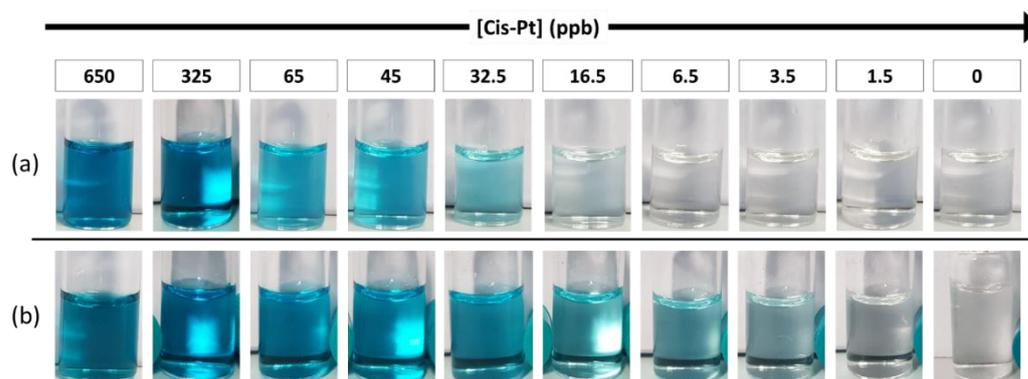
**Figure 2.** Representative colorimetric results of the assay, after 5 min color development. (a) Color change obtained at different concentrations of cisplatin (LOD ~30 ppb) in the standard configuration. (b) Colorimetric results in the enhanced configuration of the test (LOD ~3 ppb).
