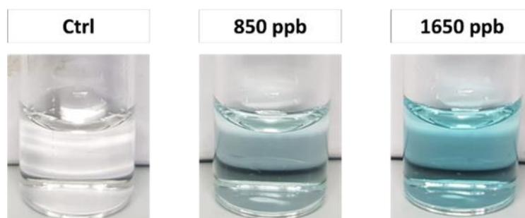
**Figure 4.** Color change obtained after 5 min at two different concentrations of cisplatin vs. negative control, in diluted synthetic urine (1:50).
