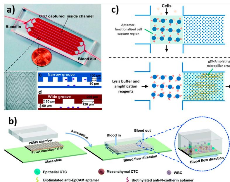
**Figure 7.** Schematic illustration of microfluidic devices for the isolation of CTCs using various techniques. (a) GEM chip with eight parallel channels with an inlet and an outlet showing asymmetric
