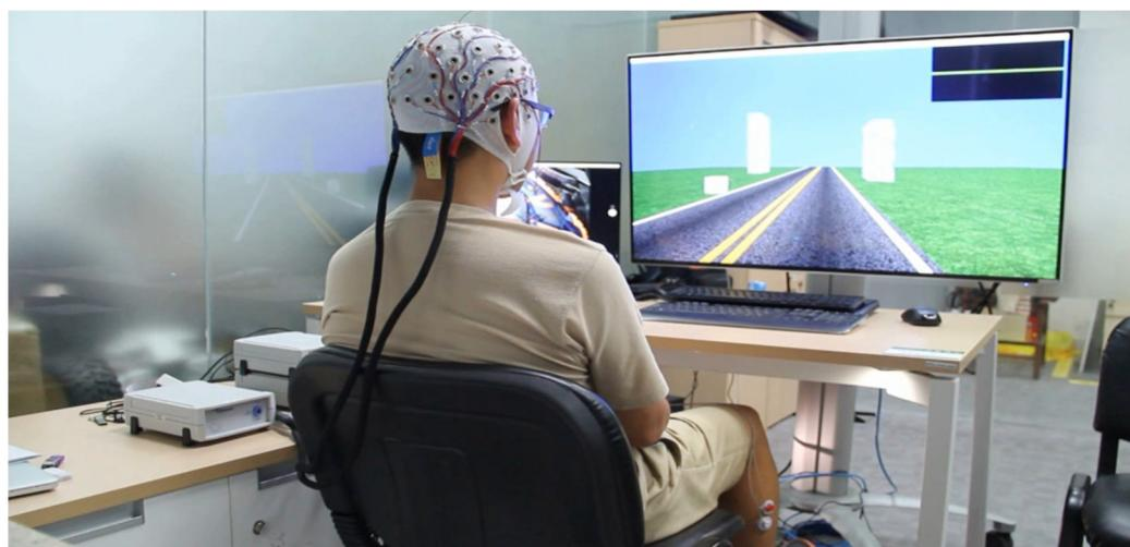
**Figure 2.** A VR-MRCP-based BCI neurorehabilitation device [47].
