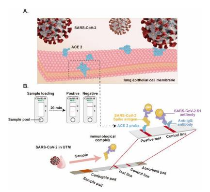
**Figure 9.** Lateral flow assay-based SARS-CoV-2 detection. (**A**), The cellular receptor of the SARS-CoV-2, the ACE2 expressed on lung epithelial cells. (**B**), Schematic of the LFIA for SARS-CoV-2 detection. Adapted from Ref. [53] with permission from Elsevier. <sup>©</sup> 2020 Published by Elsevier B.V.
