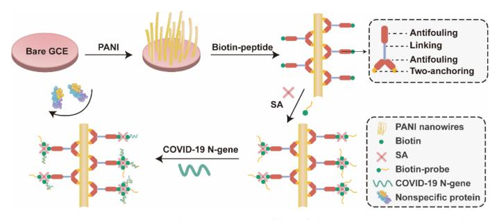
**Figure 11.** Schematic representation of the antifouling COVID-19 sensor. PANI, polyaniline; SA, streptavidin; GCE, glassy carbon electrode. Adapted from Ref. [155] with permission from the American Chemical Society. <sup>©</sup> 2021, American Chemical Society.
