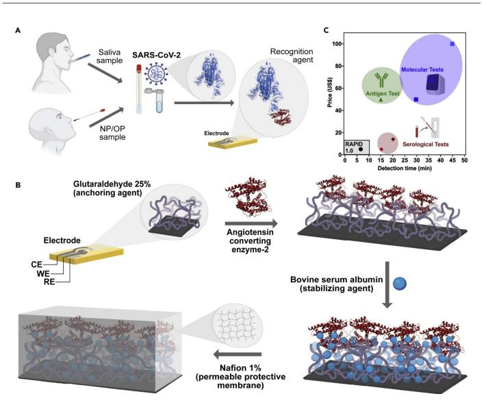
**Figure 5.** SARS-CoV-2 detection by RAPID test. (**A**), Working principle of RAPID test. (**B**), Functionalization of working electrode. (**C**), Comparison of RAPID test with some FDA-approved tests. Reprinted from Ref. [51] with permission from Elsevier. <sup>©</sup> 2021 Elsevier Inc.
