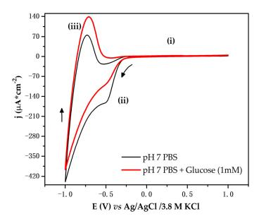
**Figure 4.** CV curves registered for the  $Ti/TiO_2$  electrode recorded at 10 mV/s in pH 7 PBS and pH 7 PBS with D(+)-glucose at 1 mM. The CV electrochemical response is characterized by region (i) where Faradaic processes do not occur. Regions (ii) and (iii) represent the reduction and oxidation process of  $TiO_2$ , respectively. Arrows depict the sense of potential sweep.
