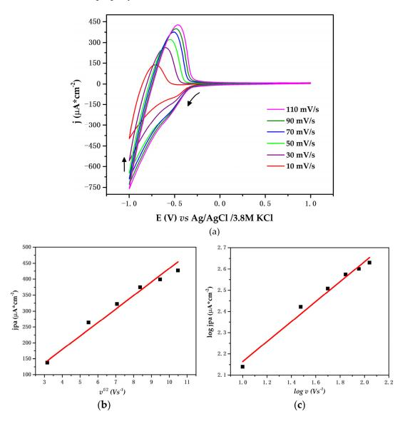
**Figure 6.** (a) CV curve of the working electrode under the effect of scan rate variation (10, 30, 50, 70, 90, and 110 mV/s), using pH 7 PBS and glucose at 1 mM. Arrows depict the sense of potential sweep. (b) Plot of anodic peak current versus square root of scan rate. (c) Plot of log anodic peak current versus log scan rate.
