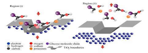
Figure 5. Proposed mechanism of interaction between ions, glucose molecules, and  $TiO_2$  grain boundaries throughout the CV process.
