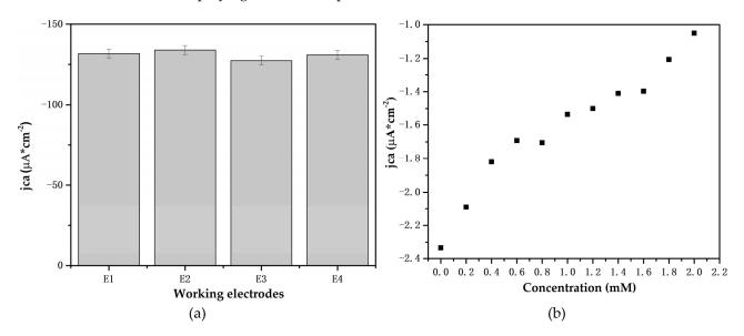
**Figure 10.** (a) Cathodic current density of the five Ti/TiO<sub>2</sub> electrodes in pH 7 PBS and glucose at 1Mm. (b) Cathodic current density of a Ti/TiO<sub>2</sub> electrode in artificial saliva solution at 330 s.
