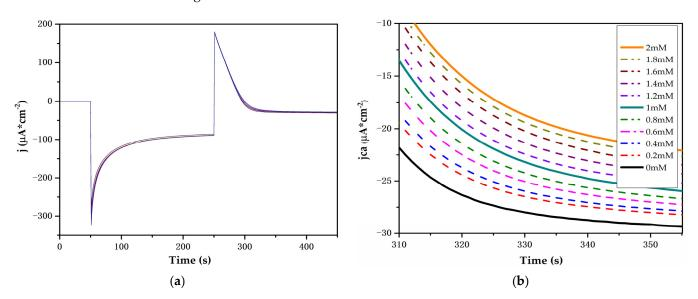
**Figure 8.** (a) Ti/TiO<sub>2</sub> electrode response to double-pulse chronoamperometry in a pH 7 PBS and glucose from 0 to 2 mM. (b) Magnification of the second chronoamperometric pulse region.
