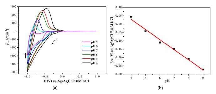
**Figure 7.** (a) Working electrode at varying pH values of PBS with glucose at 1 mM; v = 10 mV/s. Arrows depict the sense of potential sweep. (b) Relationship between cathodic potential vs. pH.
