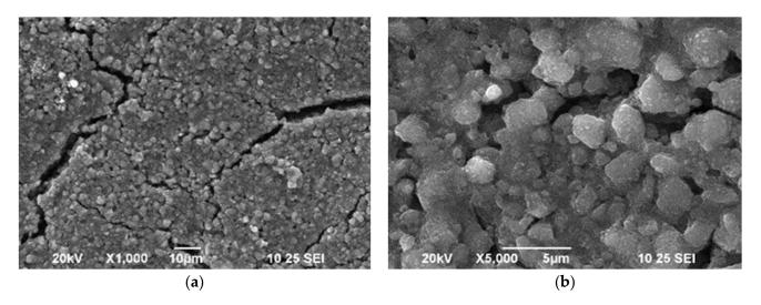
**Figure 1.** Morphology of the Ti/TiO<sub>2</sub> electrode with under (a)  $\times 1000$  and (b)  $\times 5000$  magnification.
