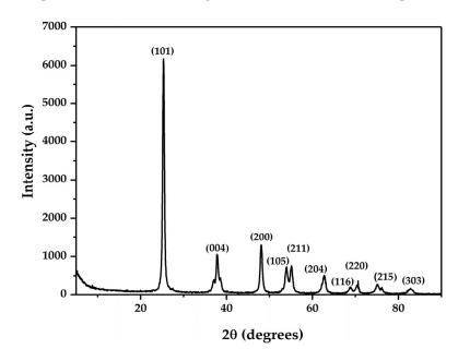
Figure 3. X-ray diffraction pattern of the Ti/TiO<sub>2</sub> electrode synthesized by spin coating.
