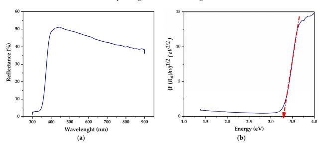
**Figure 2.** (a) Diffuse reflectance spectrum; (b) relation of  $(F(R\alpha) h\nu)^{1/2}$  vs. the energy of the Ti/TiO<sub>2</sub> electrode.
