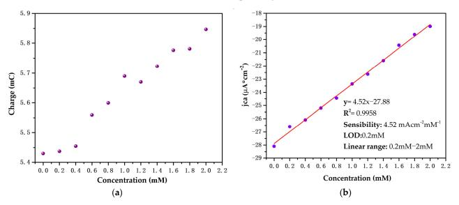
**Figure 9.** (a) Calculated charge accumulated on the electrode surface during reduction process. (b) Determination of sensitivity and limit of detection (LOD) of the synthesized electrode at 330 s.
