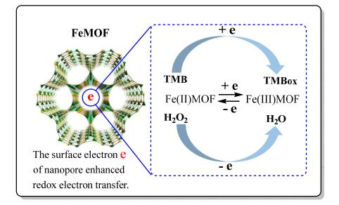
Figure 6. FeMOF nanocatalytic mechanism.
