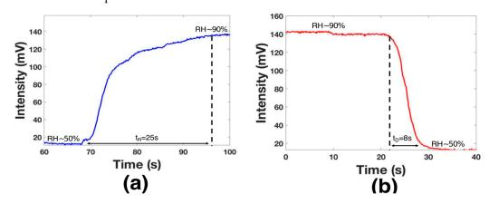
Figure 8. Analysis of the time response (a) and decay time (b).
