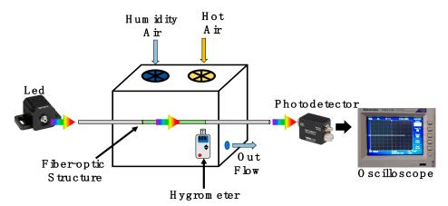
**Figure 6.** A sketch of the experimental setup used to validate the humidity response of the functionalized optical fiber sandwich structure.
