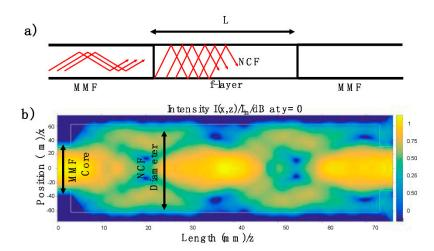
**Figure 5.** (a) Configuration of the optical fiber structure composed by an MMF and NCF; the active region is represented by the f-layer. (b) Intensity light propagation distribution through the NCF by using a launch wavelength at 522 nm.
