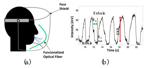
**Figure 9.** (a) Sketch of the human breath monitoring analysis; (b) voltage response of human breath monitoring using a face shield.
