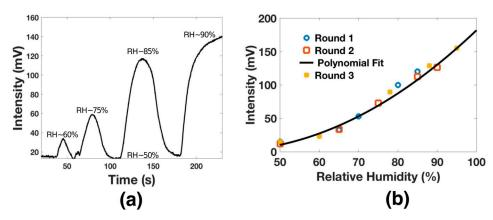
**Figure 7.** (a) The voltage output response of functionalized optical fiber for different RH. (b) Relative humidity sensitivity analysis.
