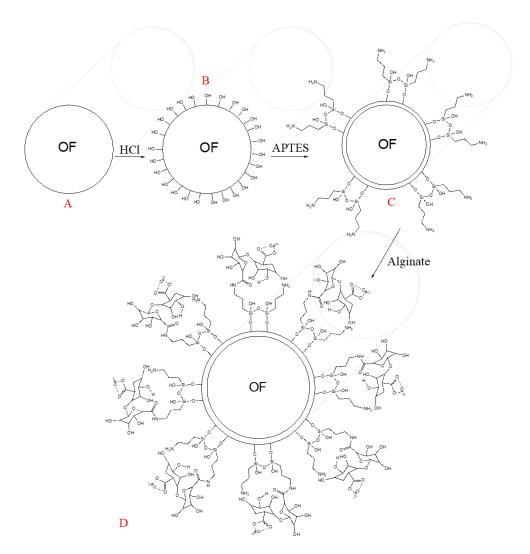
**Figure 1.** Scheme of functionalization of optical fibers with alginate. **(A)** silicon dioxide optical fiber, **(B)** hydroxyl groups formation, **(C)** APTES integration, and **(D)** calcium alginate reaction.
