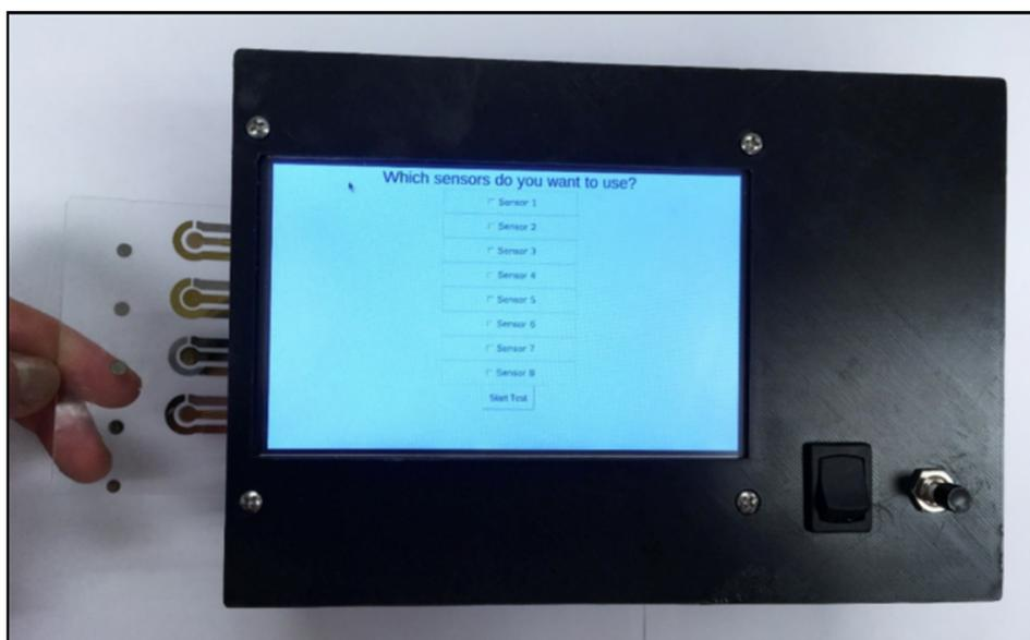
**Figure 1.** The  $\mu$ Drop system from Khetani et al. designed to perform differential pulse voltammetry to quantify C-tau and NF-L. Reprinted with permission from [36]. Elsevier 2021.
