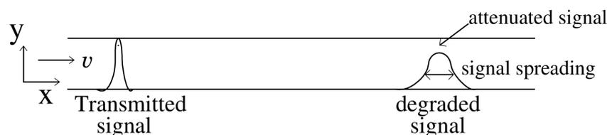
**Figure 1.** Concentration signal traversing microfluidic channel from Tx towards Rx degrades due to temporal spread and attenuation.
