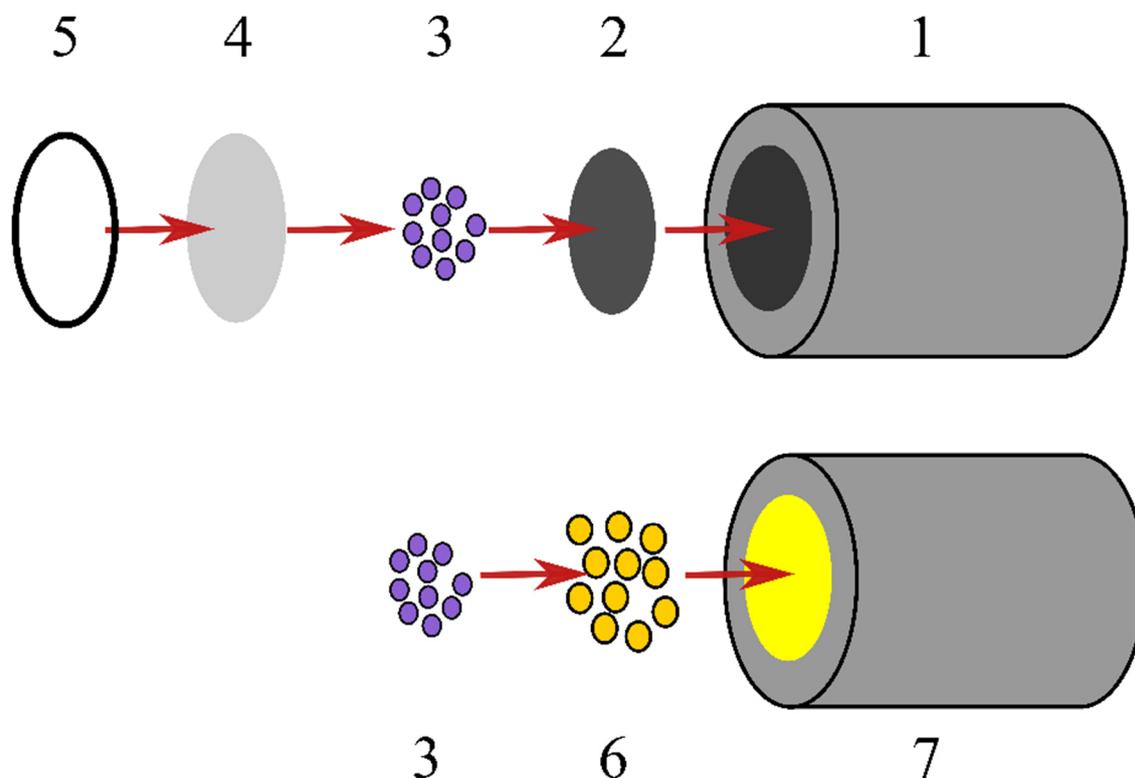
**Figure 1.** Basic scheme of the D-tagatose biosensor: 1—graphite electrode, 2—layer of TRGO, 3—layer of FDH, 4—terylene film, 5—rubber ring, 6—AuNPs modified with 4-mercaptopenzoic acid or 4-aminothiophenol, and 7—gold electrode.
