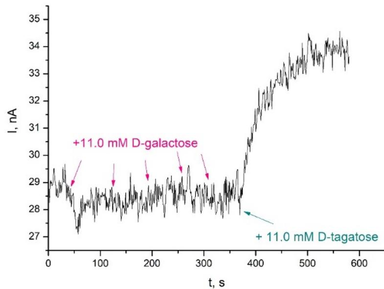
**Figure 6.** TRGO/FDH responses to D-galactose and D-tagatose. Measurement was performed in a stirred McIlvaine buffer solution, pH 4.5, 20 °C, under potentiostatic conditions (0.4 V vs. Ag/AgCl).
