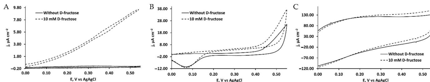
**Figure 4.** Cyclic voltammograms of AuNP/4-MBA/FDH (A), AuNP/PATP/FDH (B), and TRGO/FDH (C). Black curve—in the absence of D-fructose, and dashed curve in the presence of 10 mM D-fructose. McIlvaine buffer solution, pH 4.5, 20 °C, with a scan rate of 10 mV s<sup>−1</sup>.
