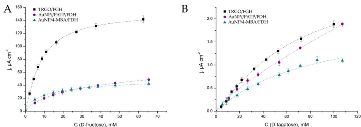
**Figure 5.** Calibration graphs for three types of sensors for changing concentrations of D-fructose (A) or D-tagatose (B). Concentrations measured under potentiostatic conditions at 0.4 V vs. Ag/AgCl in a stirred McIlvaine buffer solution, pH 4.5, 20 °C. The experimental data are fitted by using the Michaelis–Menten equation.
