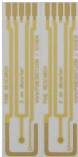
**Figure 6.** Transducer chip (gold patterned electrodes) compatible for experiment with the bridge structure, was purchased from Pine Research Instrumentation, photo taken from the pine research instrumentation website [21].
