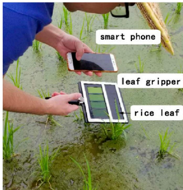
**Figure 5.** Smartphone being used to evaluate the leaf color of rice plant leaves, which is applicable in detecting nitrogen deficiencies. Reprinted with permission from [65]. ©2020 Elsevier.
